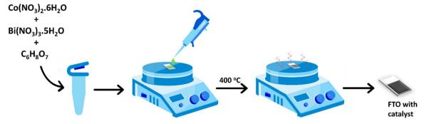
Fig. 1 Schematic of the synthesis of  $Co_aBi_bO_x$  catalysts on FTO. The procedure involves: (i) mixing Co(n) nitrate and Bi(nn) nitrate in citric acid solution, (ii) deposition of the solution onto FTO substrate, and (iii) drying and annealing the FTO-deposited metal salts.
