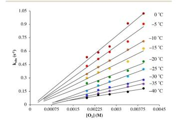
Fig. 2 Temperature-dependent rate constants  $k_{\rm obs}$  for the formation of superoxo 2 in the reaction between 1 (0.25 mM) and  $O_2$  in THF plotted against  $[O_2]$ . The intercept of approximately 0.0 would be consistent with irreversible  $O_2$  binding.
