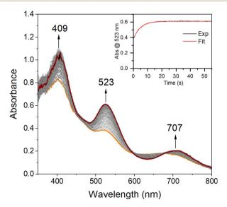
Fig. 5 Time-resolved spectral changes observed in the reaction between 3 (0.1 mM) and KO $_2$  (5.0 mM; solubilized with 222-Kryptofix) in THF at  $-40\,$  °C. Inset: kinetic trace ( $\lambda=523\,$  nm) showing the formation of 2. All reported concentrations are after mixing in the stopped-flow cell.
