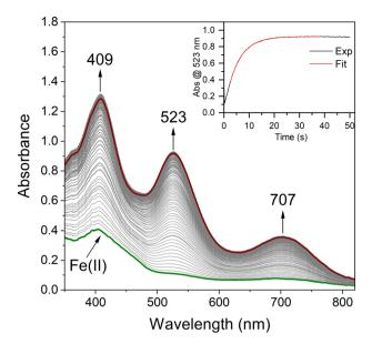
Fig. 1 Time-resolved spectral changes obtained upon mixing THF solutions of five – coordinate [Fe<sup>II</sup>( $S_2^{Me2}N_3(Pr,Pr)$ )] (1, 0.25 mM) and  $O_2$  (3.95 mM) at -40 °C. Inset: kinetic trace ( $\lambda=523$  nm) showing the formation of the Fe– $O_2$  intermediate 2. All reported concentrations are after mixing in the stopped-flow cell.
