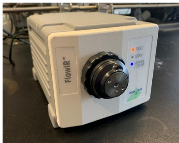
Fig. 1 Image of a FlowIR device that can be incorporated into a telescoped continuous flow sequence.
