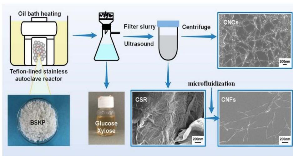
Fig. 2 Nanocellulose was prepared by hydrolyzing with dilute sulfuric acid and mechanical fibrination.<sup>25</sup>
