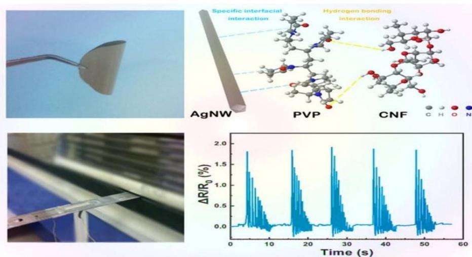
Fig. 5 AgNW/CNF hybrid nanopaper and real-time variation in the resistance of the bending sensor upon external damp vibrations.<sup>46</sup>
