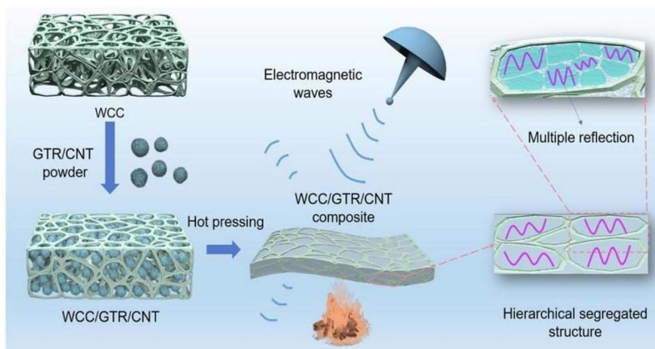
Fig. 8 Schematic diagram of the preparation of WCC/GTR/CNT composites.<sup>66</sup>
