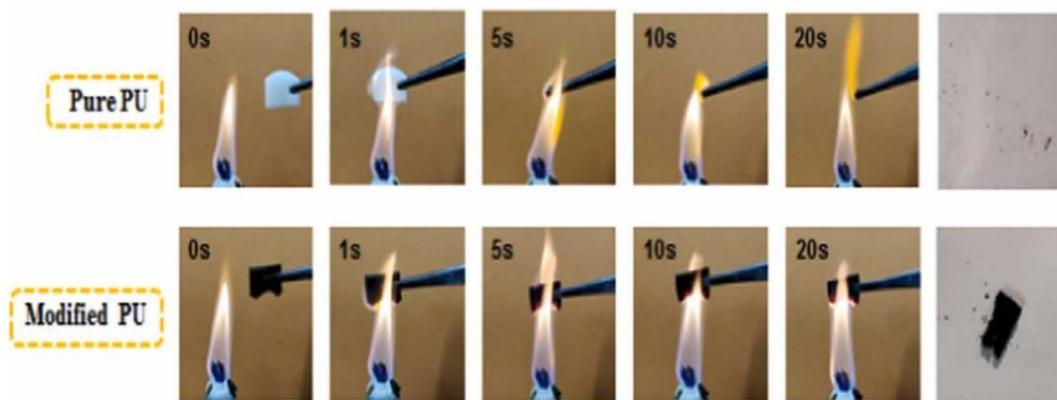
Fig. 9 Combustion process of a PU sponge.<sup>69</sup>
