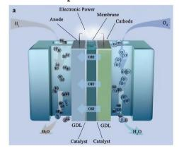
Anode: H<sub>0</sub> + 2OH = 2H<sub>2</sub>O + 2e Cathode:  $O_2 + 2H_2O + 4e^- = 4OH^-$
