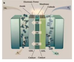
Anode: 2NH3 + 6OH- = N2+ 6H2O + 6e-Cathode:  $O_2 + 2H_2O + 4e^- = 4OH^-$
