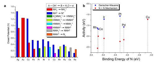
Fig. 5 (a) Onset potential investigation for different transition metals. (b) The AOR activity predicted by both mechanisms. Reproduced with permission from ref. 83 Copyright 2015, ACS publications.
