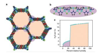
Fig. 8 The honeycomb-like channels (a) and 1D metal chain (b) of Co<sub>2</sub>Cl<sub>2</sub>btdd viewed along the z-axis. (c) Water adsorption isotherm of Co<sub>2</sub>Cl<sub>2</sub>btdd at 20 °C. Reproduced with permission from ref. 89. Copyright 2019, The Author(s)
