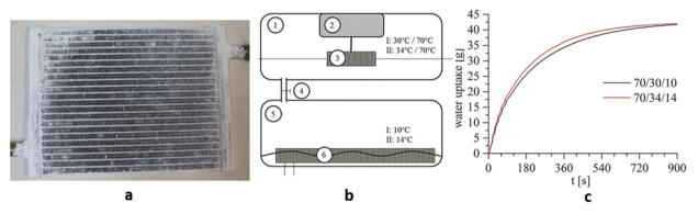
Fig. 17 (a) Image of a coated heating exchanger. (b) Schematic setup of the measurement device with 1 adsorption chamber, 2 balance, 3 adsorber with hydraulic connections, 4 valve, 5 evaporator chamber, and 6 evaporator in water with hydraulic connections. (c) Overall water uptake of the coated heating exchangers. Reproduced with permission from ref. 18. Copyright 2017, Wiley-VCH Verlag GmbH & Co. KGaA, Weinheim.
