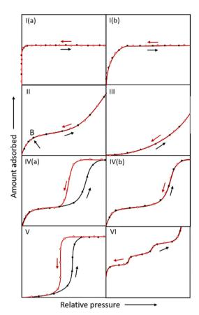
Fig. 3 IUPAC classification of adsorption isotherms. The black and red lines represent the adsorption and desorption curves, respectively.
