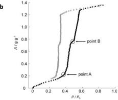
Fig. 7 (a) Structures of the MIL-100 and MIL-101. Reproduced with permission from ref. 85. Copyright 2008, American Chemical Society. (b) Water adsorption (solid symbols) and desorption (open symbols) isotherms of MIL-101 at 25 °C. Reproduced with permission from ref. 86. Copyright 2012, Elsevier Inc. All rights reserved.
