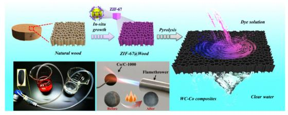
Fig. 19 Schematic diagrams of the preparation of the WC-Co composites for water treatment. Reproduced with permission from ref. 138. Copyright 2022 Elsevier B.V. All rights reserved.
