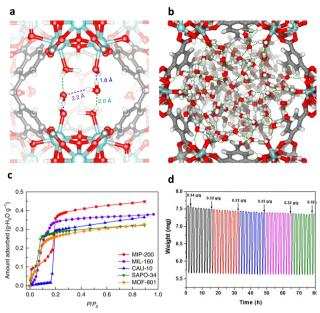
Fig. 6 (a) The initial adsorption sites for water molecules in MIP-200 at low pressure  $(P/P_0 = 0.01)$ . (b) Densely packed water molecules in the hexagonal channel at saturation ( $P/P_0 = 0.2$ ). (c) Comparison of the water adsorption isotherms of MIP-200, MIL-160, CAU-10, SAPO-34 and MOF-801 at 30 °C. (d) Thermogravimetric analysis profile for multiple cycles of water adsorption-desorption of MIP-200. Reproduced with permission from ref. 17. Copyright 2018, Springer Nature.
