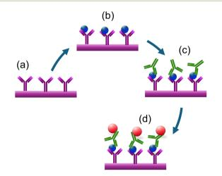
Fig. 15 The schematic representation of the magneto-nanosensor biochip immunoassay involves several steps. (a and b) Immobilization of antibodies on the surface of the working electrode. (c) Sandwich structures are formed through the addition of biotinylated detection antibodies. (d) Magnetic nanoparticles bound to the detection antibodies generate a stray magnetic field that results in a change in sensor resistance due to the GMR effect.<sup>72</sup>
