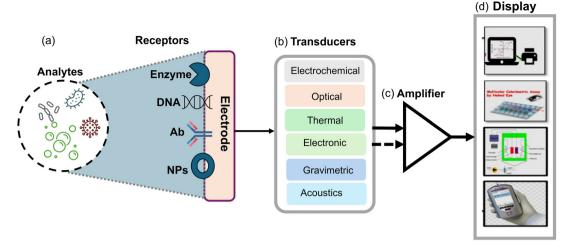
Fig. 1 Schematic diagram illustrating the operational principle of a biosensor. This includes; (a) bio-recognition elements responsible for detecting specific analytes, such as viruses, bacteria or fungi; (b and c) signal generation components like transducers and an amplifier, which converts the recognized signals into a measurable data and; (d) display units that can be used to visualize the results generated by the biosensor.
