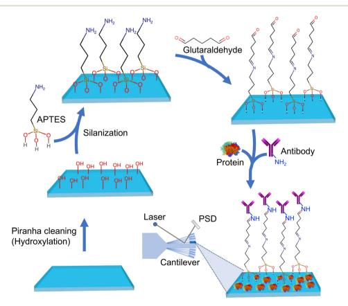
Fig. 16 Scheme showing silicon microfabricated cantilever functionalization by treating the surface with APTES, glutaraldehyde followed by colvaent attachment of anti-Aspergillus niger polyclonal antibodies ~IgG designed to capture fungal spores.<sup>73</sup> Binding of spores to the functionalized cantilever induces its deflection of the laser beam falling on it which is sensitively detected by the position sensitive detector (PSD).
