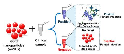
Fig. 7 Schematic illustration of the gold nanoparticle system for plasmonic detection of fungi to facilitate self-diagnosis and hygiene control of clinical fungal infections. The progression in hue from red to pink to purple to blue signifies an escalation in the concentration of fungi present in a given clinical sample.59
