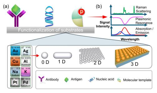
Fig. 2 (a) The functionalization process of the substrate with various optical materials and the attachment of specific receptors for enhancement of sensitivity and specificity. (b) The signal detection mechanism, involving the selection of modes such as surface plasmon resonance (SPR), absorbance, transmission or Raman scattering, enabling precise analyte detection and analysis.
