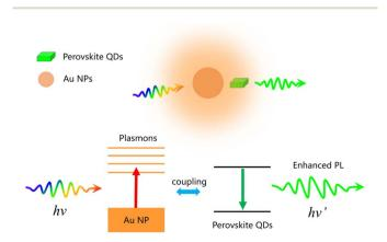
Scheme 1 Schematic illustrating the plasmonic effect on the PL performance of perovskite QDs. (upper) The near-field interactions between the Au NPs and perovskite QDs. (lower) The energy level illustration.
