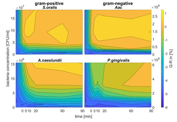
Fig. 6 Colorimetric sensing of oral bacteria species (A. naeslundii, S. oralis, Aac and P. gingivalis). G - R values of spherical CTAB-AuNP at OD<sub>AuNP</sub> 0.5 plotted as a function of incubation time.
