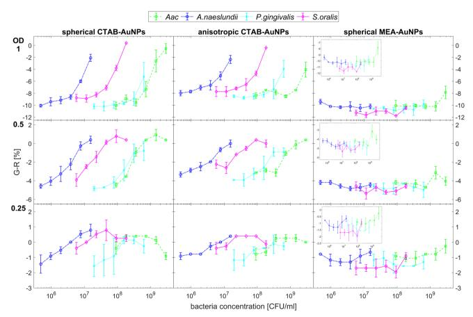
**Fig. 5** Colour change represented by average G - R values (n = 3) upon addition of bacteria to functionalized AuNPs. G - R were obtained using colorimetric assay of CTAB- and MEA-AuNPs 10 min after the addition of the respective oral bacteria (*A. naeslundii*, *S. oralis*, *Aac* and *P. gingivalis*). Error bars denote the standard deviation. Note that *y*-axes have different range for different AuNP dilutions to highlight the differences in G - R as a function of bacteria concentration.
