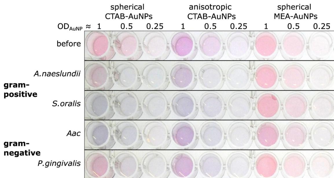
Fig. 4 A representative image of wells containing a dispersed solution of CTAB- and MEA-AuNPs (AuNP dilution in terms of  $OD_{AuNP}$  are specified on top of the well plate) before and 10 min after the addition of oral bacteria (*A. naeslundii*, *S. oralis*, *Aac* and *P. gingivalis*) at bacteria OD listed in Table 2. Due to the differences in bacteria concentration, the relative colour changes among the species cannot be compared to each other.
