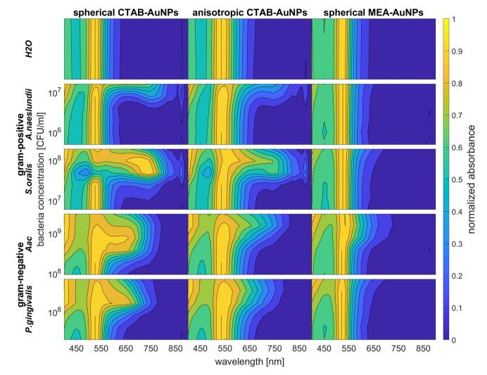
Fig. 7 Normalized absorbance values obtained via UV-vis spectroscopy of CTAB- and MEA-AuNPs at OD<sub>AuNP</sub> 0.5 measured 90 min after the addition of oral bacteria species (*A. naeslundii*, *S. oralis, Aac* and *P. gingivalis*) and water as a reference.
