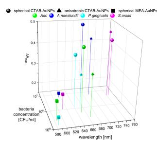
Fig. 8 Maximum absorbance change,  $\Delta A_{max}$  derived from UV-vis spectrometry of AuNPs at OD 0.25 and bacteria concentration saturation point, 90 min after the addition of oral bacteria.
