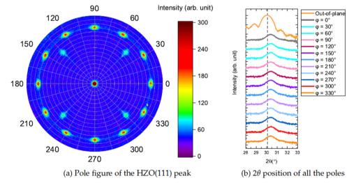
Fig. 4 Panel (a) shows the pole figure of the HZO (111) peak of a 10 nm HZO film on a single crystal STO substrate. The radial angle γ ranges from 0° up to 85° and the azimuthal angle  $\phi$  ranges from 0° to 359°. Panel (b) shows the  $2\theta$  position of each pole. The dashed line is drawn at the position of the outof-plane (111) pole as a guide to the eye.
