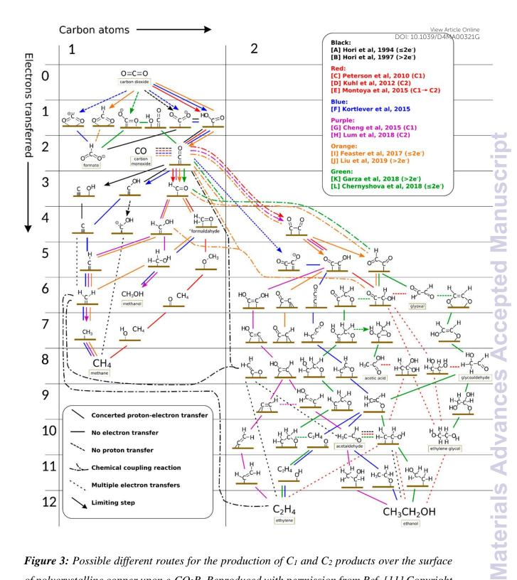
*Figure 3:* Possible different routes for the production of  $C_1$  and  $C_2$  products over the surface of polycrystalline copper upon e-CO<sub>2</sub>R. Reproduced with permission from Ref. [11] Copyright 2023, American Chemical Society.
