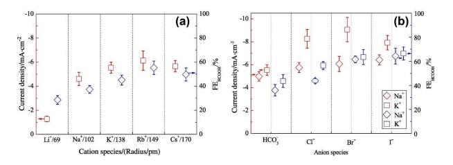
**Figure 37**: Current density and  $FE_{HCOOH}$  as functions of electrolyte type and the cation size, measured using an SnO<sub>2</sub>/C electrode at -1.4 V in (a)  $0.1 \text{ molL}^{-1}$  MHCO<sub>3</sub> ( $M = Li^+$ , Na<sup>+</sup>, K<sup>+</sup>, Rb<sup>+</sup>, Cs<sup>+</sup>) and NaX and KX ( $X = HCO_3^-$ , Cl<sup>-</sup>, Br<sup>-</sup> and I<sup>-</sup>), respectively. Reproduced with permission from Ref. [413] Copyright 2020, Elsevier.
