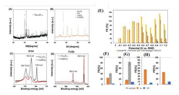
*Figure 13:* The p-XRD patterns of the  $Cu_{51}Zr_{14}$  composite alloy (A) and  $Cu\#ZrO_2$  (B) were analyzed. The HAXPES profiles of the  $Cu_{51}Zr_{14}$  precursor alloy (black) and  $Cu\#ZrO_2$  (red) were analyzed in the Zr 3d region (C) and the Cu 2p region (D). The product distribution of e- $CO_2RR$  over  $Cu\#ZrO_2$  was quantified after 3 hours of electrolysis at a potential of -0.9 V vs RHE. The e-CO\_2RR performance was evaluated for different catalysts, including a mixture of
