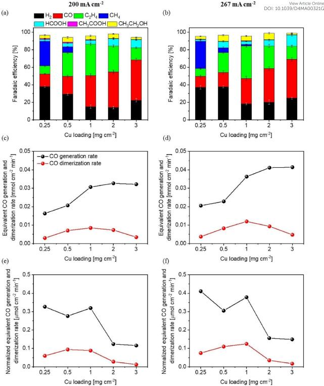
**Figure 17:** Comparison of electrodes consisting of 25 nm nanoparticles (NPs) with varying loadings: at 200 mA cm<sup>-2</sup>, (a) assessing selectivity, (c) evaluating equivalent bulk CO generation and dimerization rates, and (e) normalizing equivalent CO generation and dimerization rates to the electrode's electrochemically active surface area (ECSA); at 267 mA cm<sup>-2</sup>, (b) analyzing selectivity, (d) calculating equivalent bulk CO generation and dimerization
