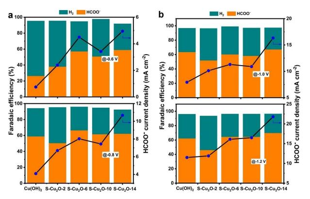
*Figure 22:* The  $FE_{HCOO}$  and partial current density were measured for  $Cu(OH)_2$ , S- $Cu_2O$ -2, S- $Cu_2O$ -6, S- $Cu_2O$ -10, and S- $Cu_2O$ -14 electrodes at various applied potentials ranging from -0.6 V to -1.2 V vs. RHE.com. Reproduced with permission from Ref. [227] Copyright 2023, Elsevier.
