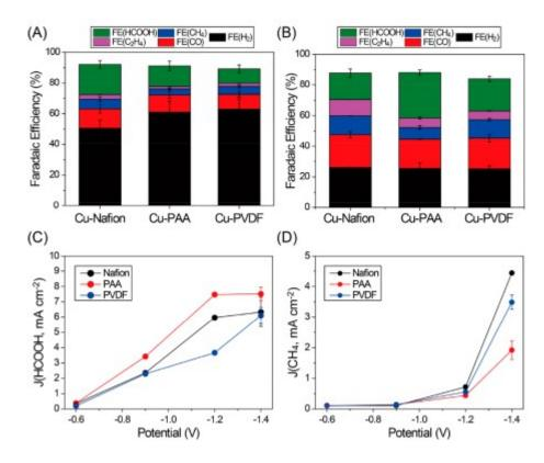
*Figure 31:* The CO<sub>2</sub>RR performance of various Cu/C catalysts with different binders was evaluated. The FE of HCOOH, CO, CH<sub>4</sub>,  $C_2H_4$ , and  $H_2$  were evaluated at two different potentials: -0.6 V and -1.4 V. The partial current density profiles of HCOOH and CH<sub>4</sub> are presented. Reproduced from Ref. [339] Open access article, American Chemical Society.
