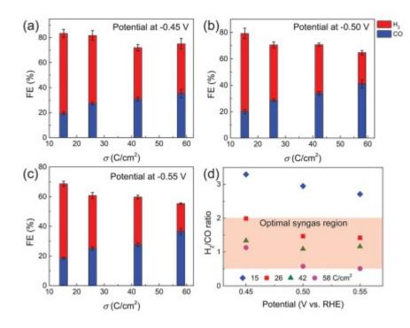
*Figure 30:* The FEs of  $H_2$  and CO production on OD-Cu NPs were measured at different applied potentials: (a) -0.45 V, (b) -0.50 V, and (c) -0.55 V. The controllable composition of syngas varies depending on both the applied potentials. Reproduced with permission from Ref. [331] Copyright 2020, American Chemical Society.
