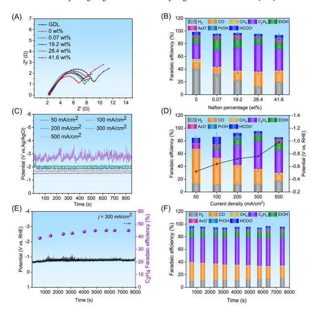
*Figure 10:* ANCu@Nafion catalysts with varying Nafion percentages were fabricated at 0.1 *V*, and their Nyquist plots from 0.01 Hz to 100 kHz (A) and their product distribution FEs at 300 mA cm<sup>-2</sup> (B) were plotted. The CO<sub>2</sub> reduction kinetics of ANCu@Nafion-28.4 wt% in 1 M KOH electrolyte (C) along with the corresponding current density versus product distribution
