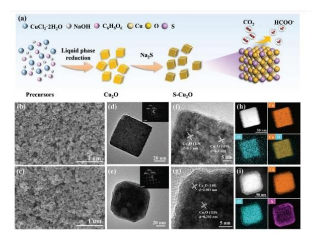
**Figure 23:** The synthesis and subsequent characterization of a particular structure. Schematic representation of the process for preparing electrocatalysts (a). The SEM images of  $S_0$ -Cu<sub>2</sub>O-70 (b) and  $S_3$ -Cu<sub>2</sub>O-70 (c) are shown. TEM images of  $S_0$ -Cu<sub>2</sub>O-70 and  $S_3$ -Cu<sub>2</sub>O-70, along with their
