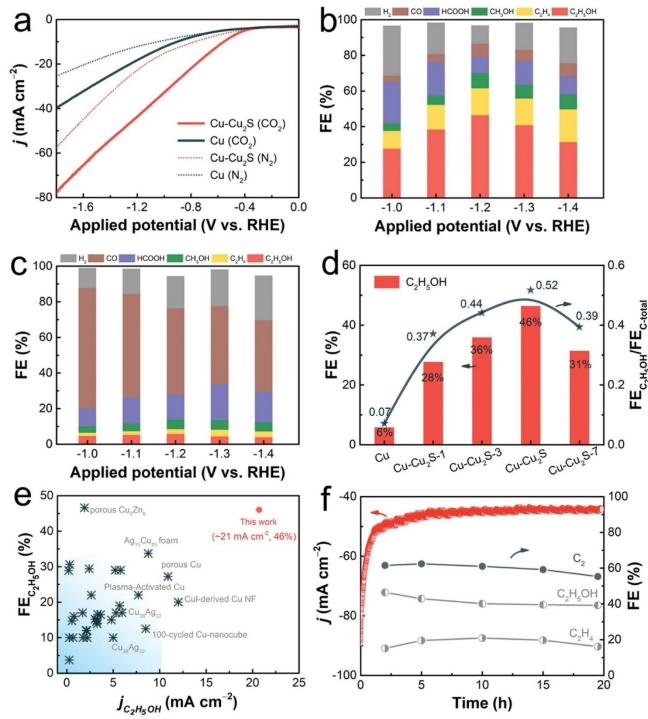
**Figure 7:** Electrochemical activity of the manufactured catalysts for  $CO_2R$ . In a  $N_2$  and  $CO_2$  saturated 0.1 M KHCO<sub>3</sub> aqueous electrolyte (a), the LSV curves of pure Cu and CuCu<sub>2</sub>S are shown. Distributions of the products of the catalyzed  $CO_2RR$  for (b) CuCu<sub>2</sub>S nanosheets and (c) pure Cu nanosheets at various applied potentials. At 1.2 V (against RHE),  $FE_{C_2H_5OH}$  and
