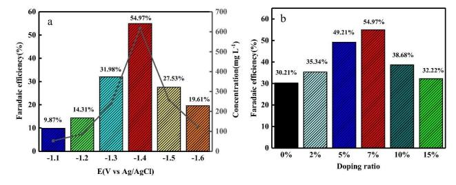
**Figure 35:** The FE of CO<sub>2</sub> reduction to formate was investigated using a carbon paper electrode loaded with 7%-(Cu, N)-SnO<sub>x</sub> at various potentials (a). The Faradaic efficiency of  $CO_2R$  to formate was studied using different electrodes with varying amounts of (Cu, N) doping at a potential of -1.4 V, with an electrolysis time of 1 hour. Reproduced with permission from Ref. [375] Copyright 2020, Elsevier.
