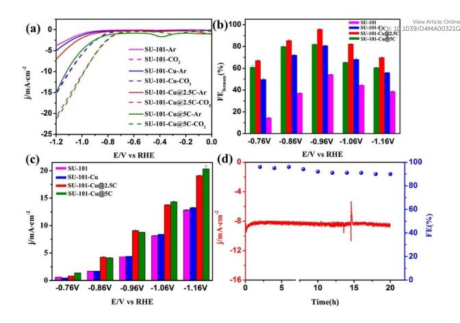
**Figure 36:** The electrocatalytic performance of SU-101, SU-101-Cu, and SU-101-Cu@xC was evaluated through LSV measurements in  $CO_2$  and Ar atmospheres (a). The measurements included different applied potentials,  $FE_{formate}$  (b), and current density (c). The SU-101-Cu@2.5C was tested for long-term durability at a voltage of -0.96 V vs RHE for a duration of 20 hours (d). Reproduced with permission from Ref. [396] Copyright 2023, Elsevier.
