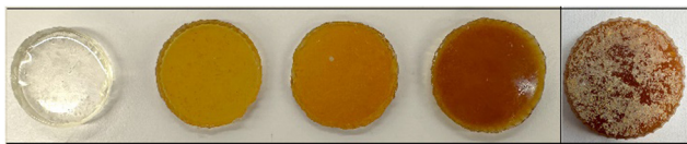
Fig. 3 Moulded discs of X -poly(siloxane- r -S). From left to right: X = 0, 5, 10, 15 wt% S and 15 wt% S after 24 h at 25 °C.
