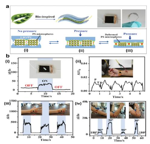
(a) Schematic illustration of the bean pod inspired healable pressure sensor and its mechanism. (b) Wearable sensing applications of the pressure sensor in the detection of (i) rice as a light object, (ii) blood pulse on the wrist, (iii) hand clenching, and (iv) elbow bending. Reproduced with permission.<sup>55</sup> Copyright 2020 American Chemical Society.
