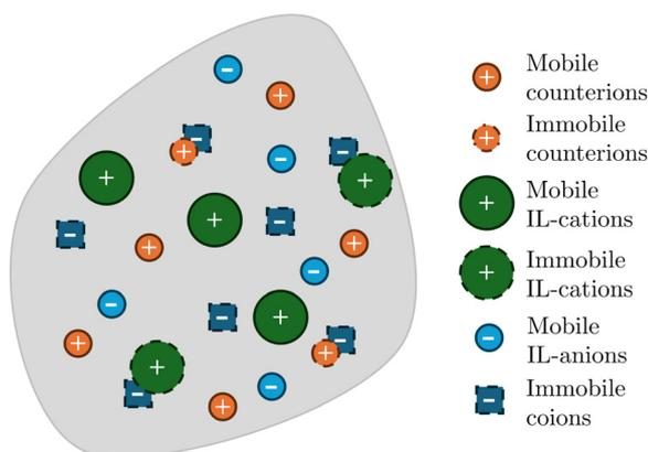
**Fig. 1** Ionic composition of IL-IPMCs modeled in this paper. Mobile and immobile ions are surrounded by solid and dashed lines, respectively. Cations in contact with fixed coions indicate immobilized cations, which do not migrate within the IL-IPMC. Note that only a fraction of counterions and IL-cations is mobile.
