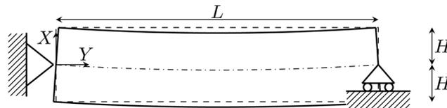
Fig. 2 Schematics of the beam-like IL-IPMC actuator.
