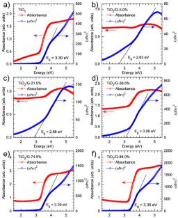
Fig. 23 UV-vis diffuse reflectance spectra and related Tauc plots of TiO<sub>2</sub> (a) and  $TiO_2$ /graphene with varying  $TiO_2$  loadings (5% (b), 21,5 (c), 36,5% (d), 74,5% (e), and 84% (f)). Reprinted with permission from ref. 131 Copyright 2021. Elsevier
