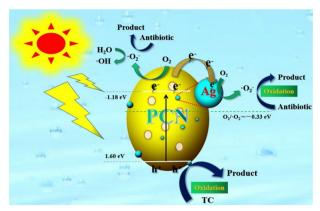
Fig. 12 Schematic illustration of photocatalytic mechanism of the Ag/ GCN plasmonic photocatalyst. Reprinted with permission from ref. 82 Copyright 2020, Elsevier.
