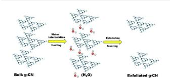
Fig. 5 Schematic illustration of the bi-thermal exfoliation method. Reprinted with permission from ref. 61 Copyright 2019, Elsevier.
