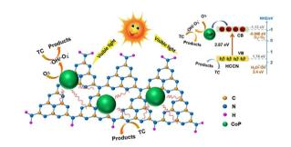
Fig. 14 Schematic illustration of CoP-modified highly crystalline g-C<sub>3</sub>N<sub>4</sub>. Reprinted with permission from ref. 90 Copyright 2020, Elsevier.
