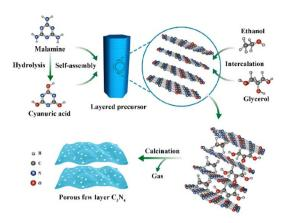
Fig. 8 Synthesis process of self-assembled porous few-layer C<sub>3</sub>N<sub>4</sub>. Reprinted with permission from ref. 65 Copyright 2019, the American Chemical Society
