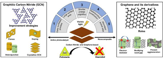
Fig. 1 Schematic illustration of the advantages of carbon nitride- and graphene-based materials for photocatalytic wastewater treatment. Graphitic carbon nitride as an active photocatalyst and its improvement strategies, with the role of graphene-based material in supporting the main photocatalyst.
