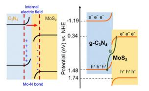
Fig. 13 Direct Z-scheme heterojunction illustration of GCN/MoS<sub>2</sub>. Reprinted with permission from ref. 84 Copyright 2023, the American Chemical Society
