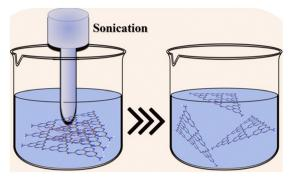
Fia. 4 Schematic illustration of the ultrasonic exfoliation method. Reprinted with permission from ref. 60 Copyright 2023, Elsevier.
