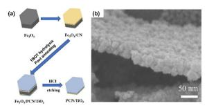
Fig. 9 (a) Illustration of Fe<sub>3</sub>O<sub>4</sub>-template assisted fabrication of PCN/TiO<sub>2</sub>. (b) SEM image of PCN/TiO2. Reprinted with permission from ref. 66 Copyright 2023, Elsevier.
