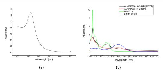
Fig. 2 (a) UV-Vis spectrum of AuNP-PEG-2K-NH<sub>2</sub>. (b) Overlayed UV-Vis spectrum of AuNP-PEG-2K-NH<sub>2</sub>(2-NIM)(DOTA), AuNP-PEG-2K-(2-NIM), Bz-DOTA and 2-NIM-COOH.
