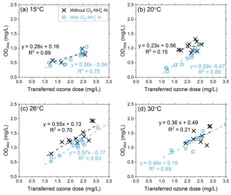
Fig. 2 Pilot-scale data depicting correlations between OD<sub>diss</sub> as a function of the transferred ozone doses at (a) 15 °C, (b) 20 °C, (c) 26 °C, and (d) 30 °C. Pilot-scale results illustrating the different Cl<sub>2</sub>-NH<sub>4</sub><sup>+</sup>-N dosing scenarios are presented in Fig. S5.†
