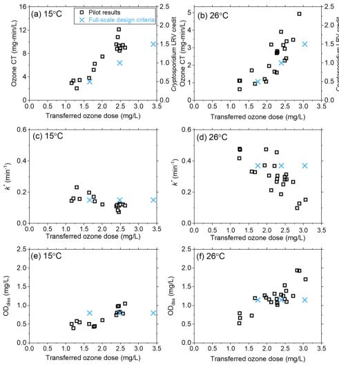
Fig. 6 Comparing pilot-scale results of this study to the initial full-scale design criteria at low (15 °C, left panels) and high (26 °C, right panels) design temperatures in terms of the effect of transferred ozone doses on (a and b) ozone CT (left y-axis) and LRV targets (right y-axis), (c and d)  $k^*$ , and (e and f)  $OD_{diss}$
