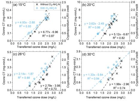
Fig. 4 Pilot-scale data depicting correlations between ozone CT (and corresponding Cryptosporidium LRV credit on the right y-axis) and the transferred ozone dose at (a) 15 °C, (b) 20 °C, (c) 26 °C, and (d) 30 °C. Fitting equations are associated with the left y-axis (ozone CT). Pilot-scale results illustrating the different Cl<sub>2</sub>-NH<sub>4</sub><sup>+</sup>-N dosing scenarios and demonstrating OD<sub>CT</sub> calculations are presented in Fig. S9.†
