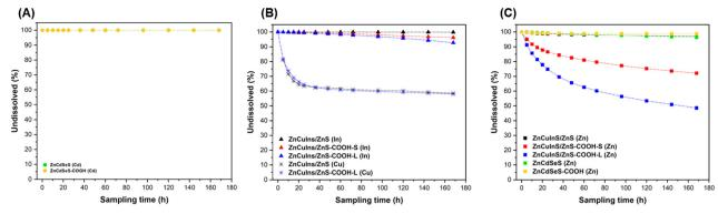
Fig. 1 Time-dependent dissolution kinetics of quantum dots (QDs) in PSF. (A) Cd-based comparison, (B) In- and Cu-based comparison and (C) Zn-based comparison. The color codes indicate the QD identity whereas different symbols are used to indicate the different ion dissolution kinetics: • = cadmium, \* = copper, ▲ = indium and ■ = zinc. All dissolution experiments were done in duplicate with an average standard deviation at each sampling point of 1-3%.
