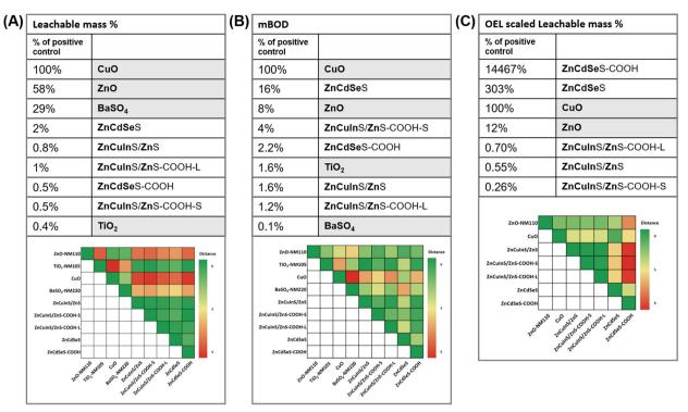
Fig. 4 Ranking and similarity analysis on three selected descriptors. All similarity plots show Euclidean distance. A) Leachable mass % after one week dissolution in PSF, all components added; B) reactivity by the FRAS assay as mass-based oxidative damage at 1 g L<sup>-1</sup>; C) leachable mass of each element scaled by its respective OEL. In all cases, CuO and ZnO serve as positive controls, whereas BaSO<sub>4</sub> and TiO<sub>2</sub> as negative controls.
