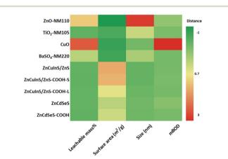
Fig. 5 Heatmap showing similarities based on assay descriptors (leachable mass % and mBOD) and intrinsic physicochemical properties (size and surface area). The legend color bar represents the association between the descriptors and the AdMa. Here red indicates an increase in assay descriptors and intrinsic physicochemical property values compared to the mean for QDs and reference materials, and green indicates a decrease in these values compared to the mean.
