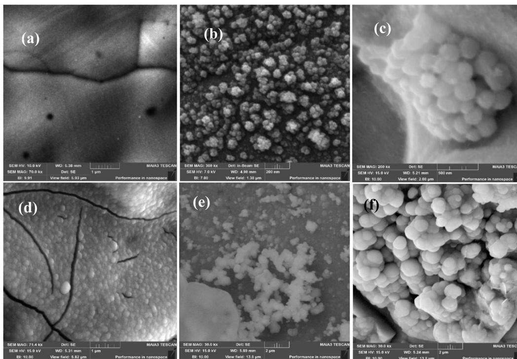
Fig. 1 SEM images of NF (a),  $\text{Mn}_2(\text{CO}_3)_3/\text{NF}$  (b),  $\text{Fe}_2(\text{CO}_3)_3/\text{NF}$  (c),  $\text{Co}_2(\text{CO}_3)_3/\text{NF}$  (d),  $\text{Ni}_2(\text{CO}_3)_3/\text{NF}$  (e),  $\text{Cu}(\text{CO}_3)/\text{NF}$  (f).
