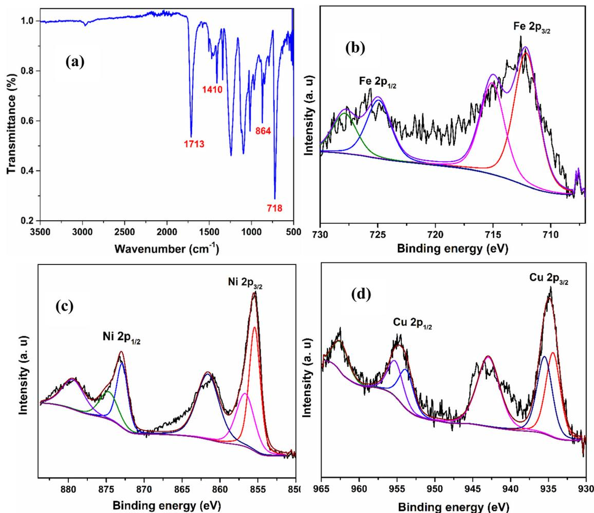
Fig. 2 ATR spectrum of  $\text{Mn}_2(\text{CO}_3)_3$  (a), XPS spectra of Fe 2p for  $\text{Fe}_2(\text{CO}_3)_3/\text{NF}$  (b), Ni 2p for  $\text{Ni}_2(\text{CO}_3)_3/\text{NF}$  (c) and Cu 2p for  $\text{Cu}(\text{CO}_3)/\text{NF}$  (d).
