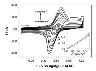
Fig. 3 Cyclic voltammograms of compound 4 recorded in DCM with the addition of tetrabutylammonium hexafluorophosphate (TBAPF<sub>6</sub>). Inset: Dependencies of anodic peak current vs. square root of scan rate. Experimental conditions:  $C_{\text{compound}} 4 = 0.1 \text{ mM}$ ,  $C_{\text{TBAPF}_6} = 50 \text{ mM}$ , glassy carbon disk electrode ( $\varnothing = 3 \text{ mm}$ );  $T = 21 \,^{\circ}\text{C}$ .
