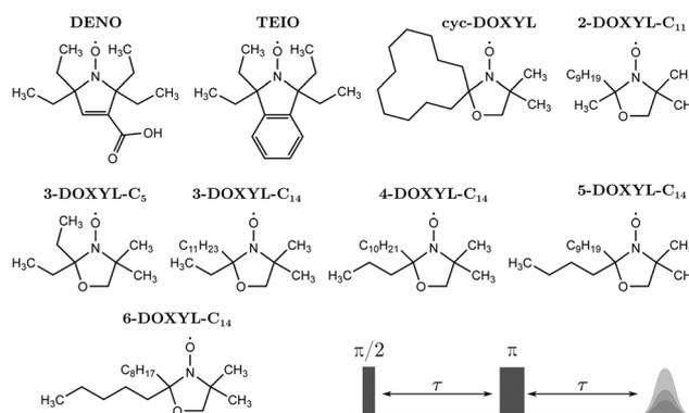
**Fig. 3** Investigated nitroxides and Hahn echo pulse sequence. Molecular structures of the pyrroline-based nitroxides containing four geminal ethyl groups *gem*-diethyl-nitroxide (DENO) and tetraethylisindoline (TEIO) and all investigated DOXYL-based nitroxides with varying alkyl chain lengths. The variable delay Hahn echo decay, *i.e.* two-pulse ESEEM, pulse sequence is illustrated schematically.
