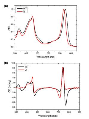
Fig. 6 (a) UV-Vis absorption spectra and (b) CD spectra for WT (black) and bchQ (red), respectively, measured at room temperature.
