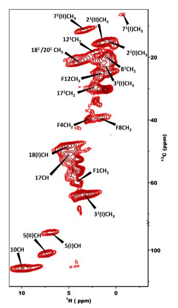
Fig. 3 2D dipolar hCH spectrum obtained at 1.2 GHz with the sample in a 1.3 mm rotor spinning at 60 kHz at a sample temperature of 277 K.
