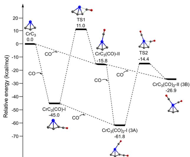
Fig. 4 Potential energy profiles of the CrC<sub>3</sub> + 2CO → CrC<sub>3</sub>(CO)<sub>2</sub> reaction calculated at the B2PLYPD3//BLYP-D3(BJ)/def2-TZVPP level of theory. Energies are given in kcal mol<sup>-1</sup>. All the molecules are in a quintet state.
