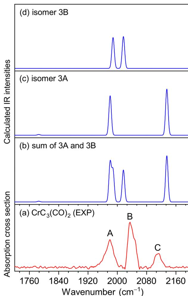
Fig. 1 Comparison of the experimental and calculated IR spectra of neutral  $\text{CrC}_3(\text{CO})_2$ . (a) Experimental IR spectrum of  $\text{CrC}_3(\text{CO})_2$ . (b) The simulated total IR spectrum of a 1 (3A):1 (3B) mixture of isomers and (c and d) simulated IR spectrum of each individual isomer calculated at the BLYP-D3(BJ)/def2-TZVPP level of theory, with the harmonic vibrational frequencies scaled by 0.991.
