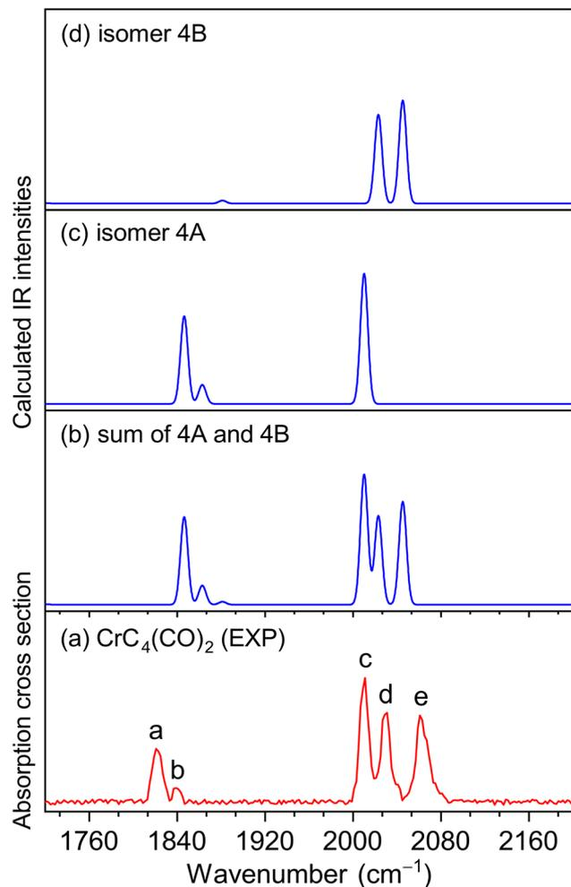
Fig. 2 Comparison of the experimental and calculated IR spectra of neutral  $\text{CrC}_4(\text{CO})_2$ . (a) Experimental IR spectrum of  $\text{CrC}_4(\text{CO})_2$ . (b) The simulated total IR spectrum of a 1 (4A):1 (4B) mixture of isomers and (c) and (d) simulated IR spectrum of each individual isomer calculated at the BLYP-D3(BJ)/def2-TZVPP level of theory, with the harmonic vibrational frequencies scaled by 0.991.
