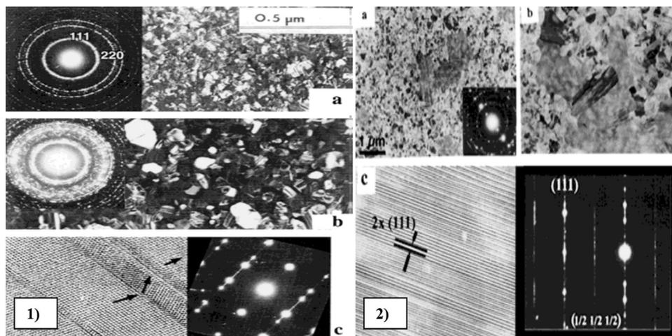
Fig. 9 TEM images of (1)  $\text{Cd}_{0.48}\text{Zn}_{0.52}\text{Te}$  thin films: (a) as-deposited state, (b) after *in situ* annealing for 15 min at 250 °C, and (c) HRTEM images. (2) *In situ*  $\text{Cd}_{0.48}\text{Zn}_{0.52}\text{Te}$  thin films annealed at 250 °C for (a) 30 min and (b) 33 min and (c) HRTEM images. Reproduced from ref. 89 with permission, Copyright (2002), Wiley-VCH.
