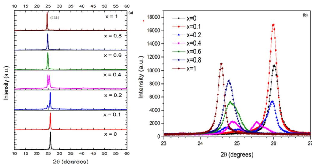
Fig. 6 (a) XRD patterns of Cd<sub>1-x</sub>Zn<sub>x</sub>Te thin films at varying Zn concentrations and (b) enlarged portion of the diffractograms in  $2\theta$  range of 23–27°, showing the position of the dominant peak. Reproduced from ref. 119 with permission, Copyright (2020), Elsevier Ltd.
