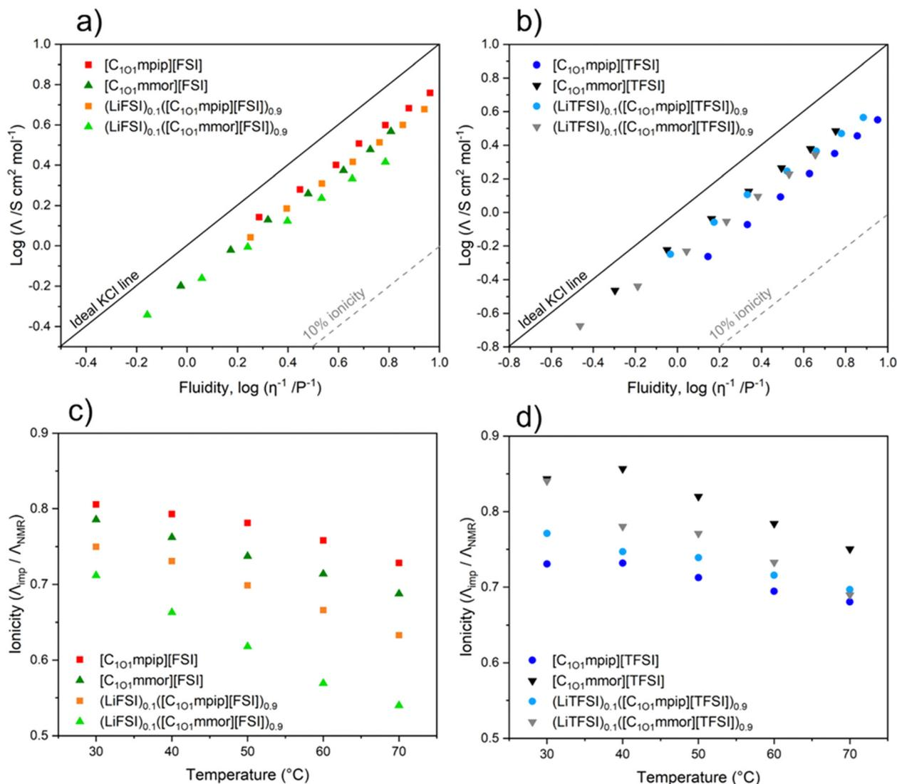
Fig. 7 Walden plot for (a) FSI-based ILs and their electrolyte solutions and (b) TFSI-based ILs and their electrolyte solutions, where  $\Lambda$  is molar conductivity calculated from experimental impedance data and  $\eta^{-1}$  is fluidity, and temperature-dependant ionicity  $I_{\text{HR}}$  of (c) FSI-based ILs and their electrolytes and (d) TFSI-based ILs and their electrolytes. Errors were calculated at  $<4\%$  for all ionicity measurements.
