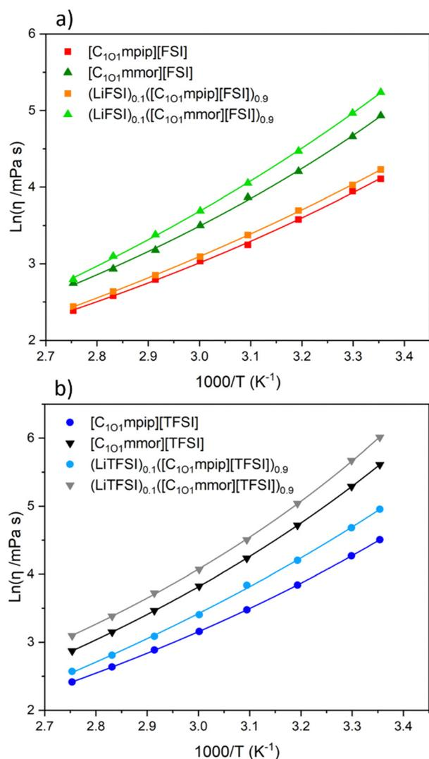
Fig. 4 Temperature dependent viscosity plots of (a) FSI-based ionic liquids and their 10 mol% LiFSI electrolyte solutions and (b) TFSI-based ionic liquids and their 10 mol% LiTFSI electrolyte solutions.
