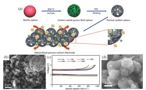
Fig. 6 (a) Schematic illustration of the synthesis processes of PCS. (b) SEM images of PCS; The inset is a high magnification SEM image of the PCS. (c) Cycling at 2.0 A g<sup>-1</sup> while curtailing the capacity to 1000 mA h g<sup>-1</sup> and (d) SEM image of discharged PCS electrode. (Reproduced from ref. 76 with permission from the WILEY).
