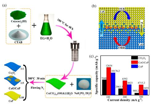
Fig. 10 (a) Synthesis process of Co<sub>3</sub>O<sub>4</sub>, CoO/CoP and CoP nanosheets. (b) "O-P interpenetration effect" in CoO/CoP heterostructured nanosheet interface. (c) The initial discharge capacity at different current densities with different electrodes. (Reproduced from ref. 15 with permission from the American Chemical Society)
