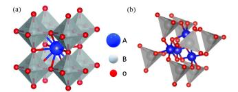
Fig. 12 (a) Crystal structures of a cubic perovskite oxide (ABO<sub>3</sub>) (reproduced from ref. 118 with permission from the Royal Society of Chemistry) and (b) a spinel oxide (AB<sub>2</sub>O<sub>4</sub>).
