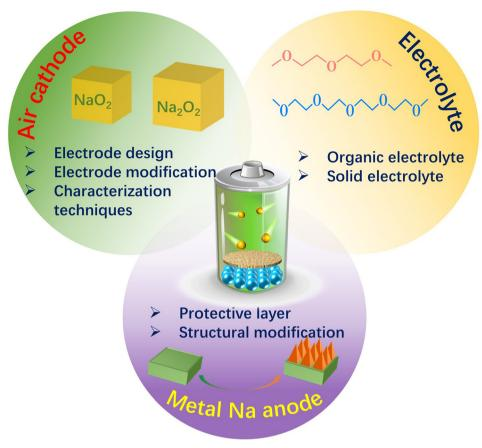
Fig. 21 The major challenges facing the development of Na-air batteries.
