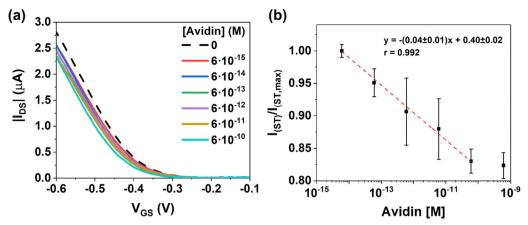
Fig. 4 (a) Transfer characteristics ( $V_{DS} = -0.1$  V) of an EGOFET employing as gate electrode a CGE with collected biotin-AuMNPs previously incubated in a PBS solution of different AV concentrations. The dashed curve represents the transfer after the exposition of the CGE with collected biotin-AuMNPs to a reference PBS solution. (b) Relative  $I_{DS}$  (at  $V_{GS} = -0.6$  V) vs. AV concentration plot and the calibration.
