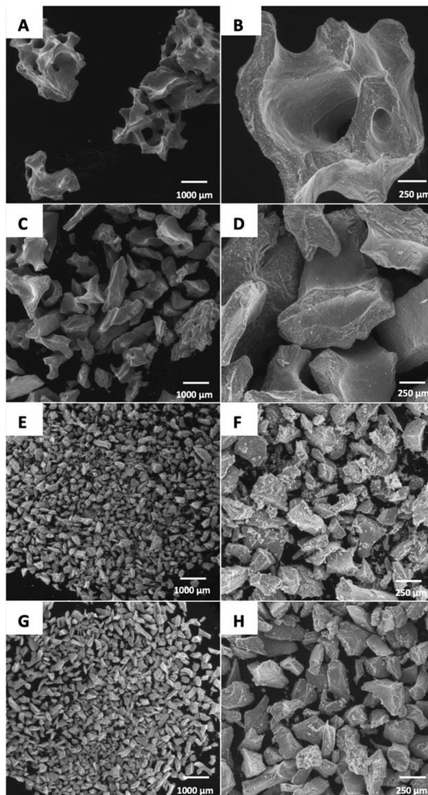
Fig. 1 SEM images of the investigated Bio-oss<sup>®</sup> granules: (A) and (B) large (BO-L); (C) and (D) small (BO-S); (E) and (F) pulverized from BO-L (BO-Lp); (G) and (H) pulverized from BO-S (BO-Sp).
