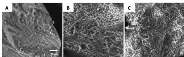
Fig. 3 High magnification SEM images of the investigated granules derived from BioOss<sup>®</sup> (A), sphene scaffolds (B) and sphene foam blocks (C).
