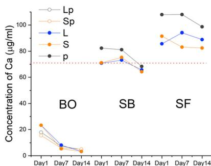
**Fig. 7** ICP-MS quantification of Ca in the cell culture medium at 1, 7 and 14 days after incubation of the biomaterials. Standard error equal to 5% for all values. BO: Bio-Oss<sup>®</sup>; SB: 3D printed sphene blocks; SF: sphene foam blocks. L: large granules; S: small granules; p: pulverized granules (Lp and Sp: pulverized from BO-L and BO-S, respectively). Red dotted line = control.
