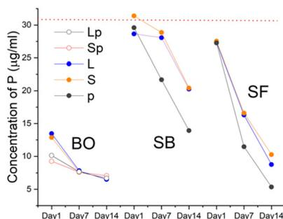
**Fig. 8** ICP-MS quantification of P in the cell culture medium at 1, 7 and 14 days after incubation of the biomaterials. Standard error equal to 10% for all values. BO: Bio-Oss<sup>®</sup>; SB: 3D printed sphene blocks; SF: sphene foam blocks. L: large granules; S: small granules; p: pulverized granules (Lp and Sp: pulverized from BO-L and BO-S, respectively). Red dotted line = control.
