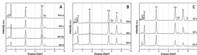
Fig. 4 EDS spectra of the investigated materials: (A) Bio-oss<sup>®</sup> (BO); (B) 3D printed sphene blocks (SB); (C) sphene foam blocks (SF). For details of acronyms see Table 1.
