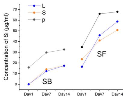
**Fig. 9** ICP-MS quantification of Si in the cell culture medium at 1, 7 and 14 days after incubation of the biomaterials. Standard error equal to 15% for all values. BO: Bio-Oss<sup>®</sup>; SB: 3D printed sphene blocks; SF: sphene foam blocks. L: large granules; S: small granules; p: pulverized granules (Lp and Sp: pulverized from BO-L and BO-S, respectively).
