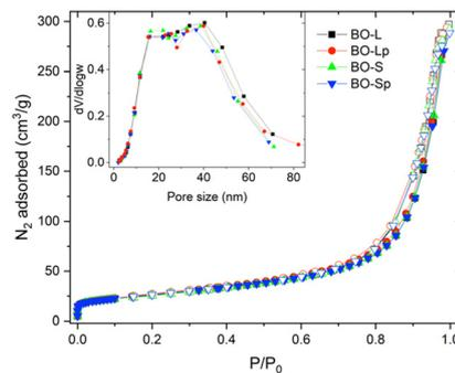
Fig. 5 Isotherms of Bio-oss<sup>®</sup> granules large (BO-L); small (BO-S); pulverized from BO-L (BO-Lp) and from BO-S (BO-Sp). Open symbols are for desorption. The inset graph represents the pore size distribution, evaluated using the BJH model in desorption.
