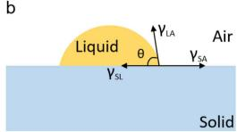
Fig. 1 (a) A schematic illustration of the interfacial absorbed NP, where R is the radius of NP. (b) Schematic illustration of a sessile droplet on a solid surface, with the relationship between the CA and surface tension  $\gamma$ . Reproduced with permission. <sup>22</sup> Copyright © 2019 Wiley-VCH GmbH.
