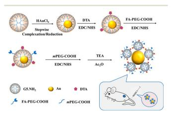
**Fig. 6** Schematic presentation of the preparation of Au DSNs-DTA-FA for targeted enhanced CT imaging of tumors. Reproduced with permission.<sup>17</sup> Copyright 2020, American Chemical Society.
