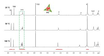
Fig. 3 qHNMR spectra (500 MHz) at different temperature of cage TP2 in TCE- $d_2$ . The green dashed rectangle highlights the appearance of a two-spin system of type AB for the aromatic protons located at C-4 and C-5 as the temperature increases. The red bars indicate the fixed integration areas for yield calculation using TBB as the internal standard. TBB = 1,3,5-tribromobenzene, TCE = 1,1,2,2-tetrachloroethane.
