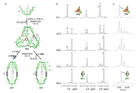
Fig. 5 Monitoring the metamorphosis reaction. (a) Schematic representation of the cage metamorphosis. (b) Sections of  $^{1}H$  NMR spectra (500 MHz, CDCl<sub>3</sub>, RT) and (c) GPC traces of the metamorphosis at different times. Time 0 hour shows the  $^{1}H$  NMR and GPC trace of TP2 assembled under reversible conditions (no molecular sieves, after 72 hours at 110  $^{\circ}C$  in CDCl<sub>3</sub>). Subsequently to t = 0 hour, THB was added.
