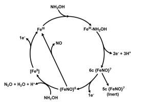
Fig. 1 The working catalytic cycle of cytochrome P460. Adapted from ref. 16.
