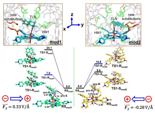
Fig. 10 The ZPE corrected QM/MM/UB3LYP/def2-TZVP reaction profile diagram along with the optimized structures and key geometric data for mod1 and mod2 cages. PES scanning for HAT has been performed for the doublet ground state of the complex. Distances are in Å, and energies are reported in kcal mol<sup>-1</sup> relative to RS. The gaussian convention is used for electric field vectors.
