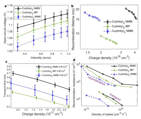
Fig. 5 Characterisation of XY1:L1-sensitised solar cells by electrolyte composition. (a) Ideality factor from open-circuit voltage *versus* light intensity. (b) Electron recombination lifetime from transient photovoltage (enlarged with errorbars in Fig. S10†) and (c) electron transport time from transient photocurrent *versus* charge carrier density. (d) Transport and recombination resistance from electrochemical impedance spectroscopy.
