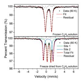
Fig. 4 (Top) Mössbauer spectrum of a flash-frozen benzene solution of 1. Fit parameters:  $\delta=0.50$  mm s<sup>-1</sup>,  $\Delta E_{\rm Q}=1.35$  mm s<sup>-1</sup>. (Bottom) Mössbauer spectrum of the same sample, after subliming away the benzene. Fit parameters:  $\delta=0.60$  mm s<sup>-1</sup>,  $\Delta E_{\rm Q}=0.80$  mm s<sup>-1</sup> (site 1, green);  $\delta=0.45$  mm s<sup>-1</sup>,  $\Delta E_{\rm Q}=2.11$  mm s<sup>-1</sup> (site 2, blue). Both spectra were recorded at 80 K.
