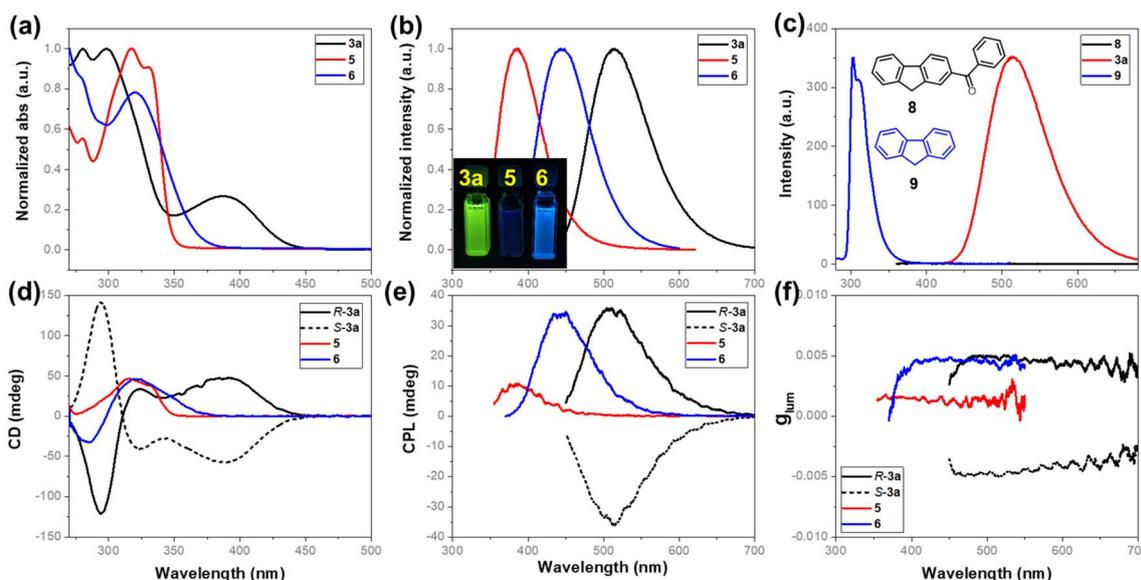
Fig. 2 (a) UV-vis and (b) fluorescence spectra of **3a**, **5**, and **6** in  $\text{CH}_3\text{CN}$ ; (c) fluorescence spectra of **3a** ( $2 \times 10^{-5}$  M), **8** ( $2 \times 10^{-5}$  M), and **9** ( $5 \times 10^{-6}$  M) in  $\text{CH}_3\text{CN}$ ; (d) ECD and (e) CPL spectra of *P*-**3a**, *M*-**3a**, **5**, and **6** in  $\text{CH}_3\text{CN}$  ( $5 \times 10^{-5}$  M); (f) luminescence dissymmetry factors  $g_{lum}$  of *P*-**3a**, *M*-**3a**, **5**, and **6**.
