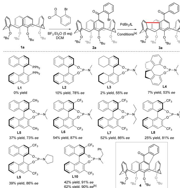
Scheme 2 Structures of ligands. [a] Sealed tube, inert atmosphere, **2a** (0.05 mmol), PdBr<sub>2</sub> (0.1 eq.), **L** (0.2 eq.), Cs<sub>2</sub>CO<sub>3</sub> (2 eq.), THF (1.5 mL), 110 °C; [b] PdBr<sub>2</sub> (0.1 eq.), **L10** (0.2 eq.), Rb<sub>2</sub>CO<sub>3</sub> (3 eq.), under otherwise standard conditions.
