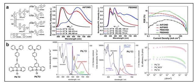
Fig. 5 Chemical structures, absorption and emission spectra, devices EQE of (a) AtFOND and PBSNND; reproduced with permission from ref. 56. Copyright 2021 Materials Advances. (b) PtL<sup>1</sup>Cl and PtL<sup>2</sup>Cl; reproduced with permission from ref. 58. Copyright 2014 Journal of Materials Chemistry C.
