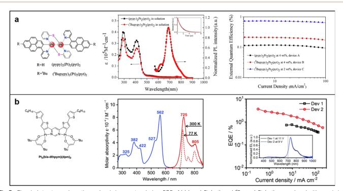
Fig. 7 Chemical structures, absorption and emission spectra, devices EQE of (a) (pypy)<sub>2</sub>Pt<sub>2</sub>(pyt)<sub>2</sub> and (<sup>t</sup>Bupypy)<sub>2</sub>Pt<sub>2</sub>(pyt)<sub>2</sub>; reproduced with permission from ref. 64. Copyright 2017 Dyes and Pigments. (b) Pt<sub>2</sub>(bis-dthpym)(dpm)<sub>2</sub>. reproduced with permission from ref. 65. Copyright 2021 Journal of Materials Chemistry C.
