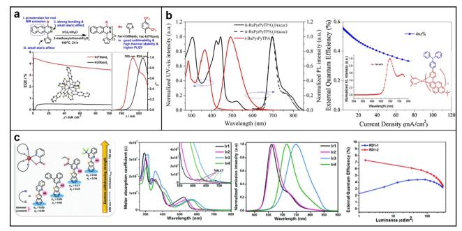
Fig. 8 Chemical structures, absorption and emission spectra, devices EQE of (a) Ir(dtbpa)<sub>3</sub> and Ir(Ftbpa)<sub>3</sub>; Reproduced with permission from ref. 67. Copyright 2017 Chemistry of Materials. (b) (t-BuPyrPyTPA)2Ir(acac); reproduced with permission from ref. 68. Copyright 2018 Chemical Physics Letters. (c) Quinoline-based Iridium(III) complexes Ir1-Ir4. Reproduced with permission from ref. 69. Copyright 2020 Journal of Materials Chemistry C.
