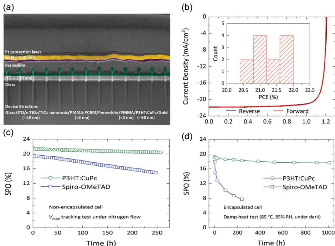
Fig. 10 (a) Cross-sectional SEM image, (b)  $J$ - $V$  performance and (c) SPO of nonencapsulated cells based on P3HT:CuPc and spiro-OMeTAD HTL measured by  $V_{mpp}$  tracking under continuous 1 Sun illumination intensity. (d) SPO of encapsulated cells based on P3HT:CuPc and Spiro-OMeTAD HTL. Reproduced with permission.<sup>131</sup> Copyright 2021, Science.
