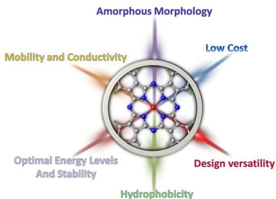
Fig. 12 Required characteristics of Pcs for minimizing the defects in perovskites or on their surface, enhancing their interfacial contact with the active layer and inhibiting the incursion of moisture.
