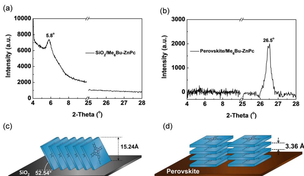
Fig. 7 GIXRD patterns of Me<sub>6</sub>Bu-ZnPc deposited on (a) SiO<sub>2</sub> and (b) perovskite (thin film thickness of ~60 nm). Molecular orientation model of Me<sub>6</sub>Bu-ZnPc deposited on (c) SiO<sub>2</sub> and (d) perovskite. Reproduced with permission.<sup>100</sup> Copyright 2019, Wiley.
