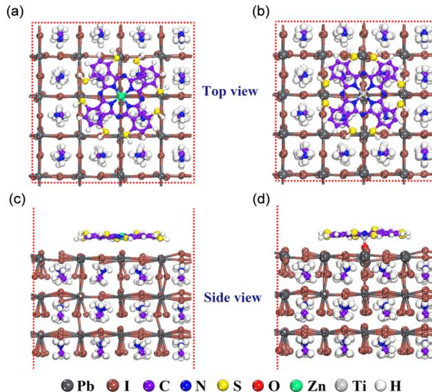
Fig. 11 (a) Top and (b) side views of  $\text{MAPbI}_3/\text{NP-SC}_6\text{-ZnPc}$ . (c) Top and (d) side views of  $\text{MAPbI}_3/\text{NP-SC}_6\text{-TiOPc}$  for relaxed structures by DFT calculation. Reproduced with permission.<sup>150</sup> Copyright 2021, Wiley.
