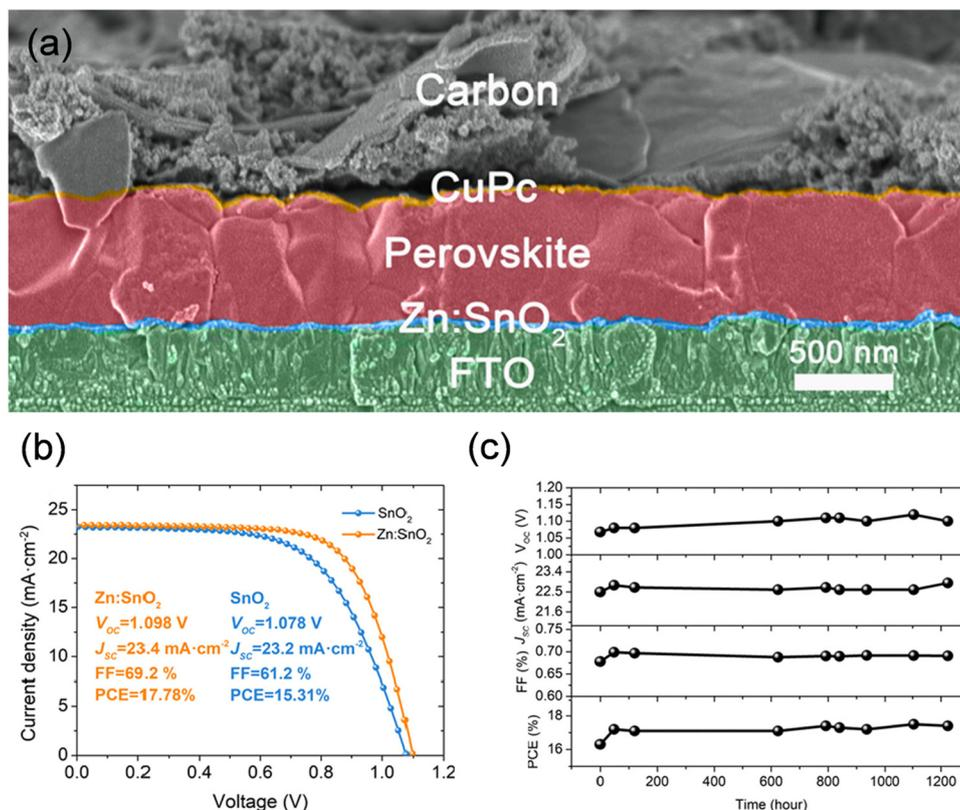
Fig. 2 (a) High-resolution cross-sectional SEM image of the carbon-based planar-structured PSC, (b)  $J$ - $V$  curves of the best-performing PSC with SnO<sub>2</sub> or Zn-doped SnO<sub>2</sub> as the ETM, (c) and evolution of the  $J$ - $V$  parameters of the Zn-doped SnO<sub>2</sub>-based devices stored in the ambient air with a relative humidity of ~20%. Reproduced with permission.<sup>64</sup> Copyright 2019, Elsevier.
