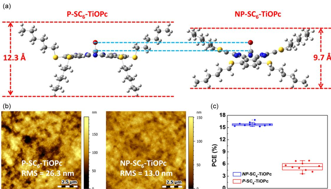
Fig. 8 (a) DFT results of the side view of the P-SC<sub>6</sub>-TiOPc- and NP-SC<sub>6</sub>-TiOPc-optimized ground state geometry (Gaussian 09 optimization with DFT B3LYP/6-31g(d)). (b) AFM images of P-SC<sub>6</sub>-TiOPc deposited and NP-SC<sub>6</sub>-TiOPc deposited on perovskite. (c) PCE statistics of devices fabricated from the same batch. Reproduced with permission.<sup>103</sup> Copyright 2019, ACS.
