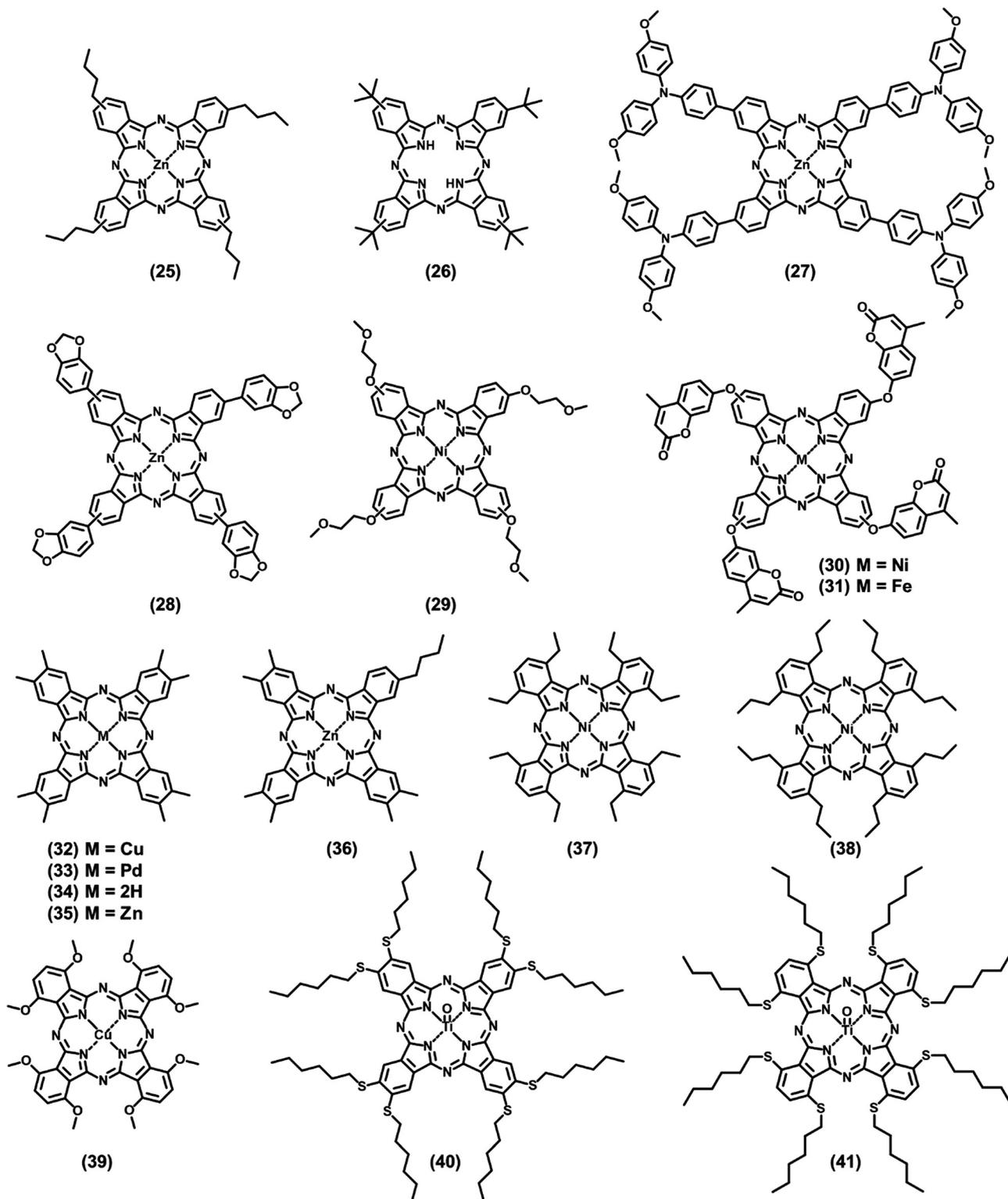
Fig. 3 Molecular structures of Pc-based dopant-free HTMs (1–41).
