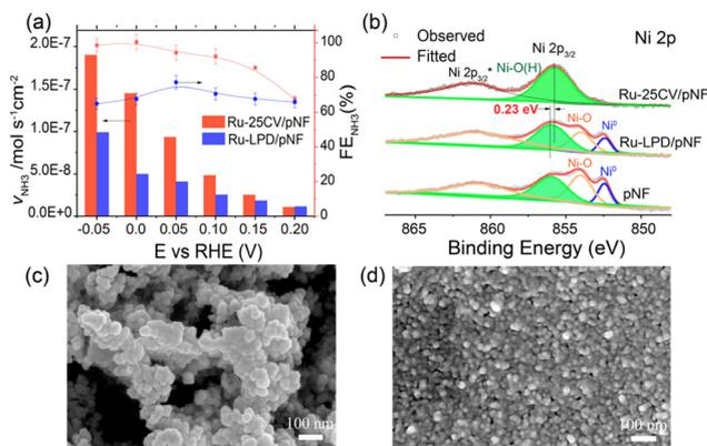
**Fig. 2** (a) The ammonia yield rate ( $V_{\text{NH}_3}$ ) and ammonia current faradaic efficiency ( $\text{FE}_{\text{NH}_3}$ ) of Ru-LPD/pNF and Ru-25CV/pNF, measured in  $1.0 \text{ M KOH}$  with  $1.0 \text{ M NaNO}_3$ . (b) The XPS Ni 2s spectra of the Ru-LPD/pNF and Ru-25CV/pNF. The SEM images of (c) Ru-LPD/pNF and (d) Ru-25CV/pNF.
