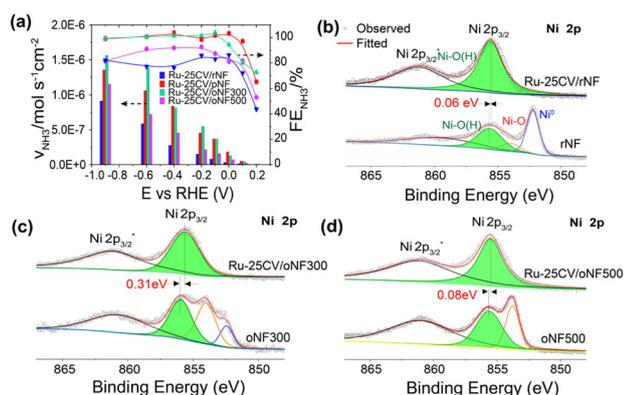
**Fig. 5** (a) The ammonia yield rate ( $V_{NH_3}$ ) and ammonia current faradaic efficiency ( $FE_{NH_3}$ ) for Ru-25CV on different NF, measured in Ar saturated-1.0 M KOH with 1.0 M NaNO<sub>3</sub> at the scan rate of 10 mV s<sup>-1</sup>. The XPS Ni 2s spectra of (b) the Ru-25CV/rNF and rNF, (c) the Ru-25CV/oNF300 and oNF300, and (d) the Ru-25CV/rNF and rNF.
