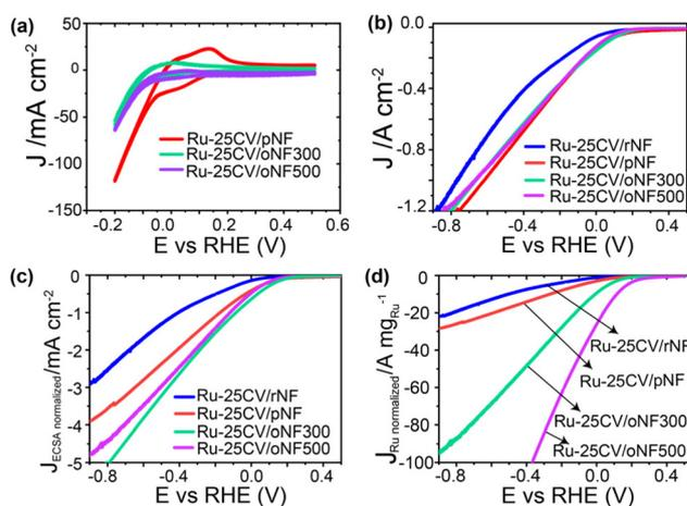
**Fig. 4** (a) The LSV of electrodes in Ar saturated 1.0 M KOH. The (b) original, (c) the ECSA normalized and (d) the Ru amount normalized LSV of Ru-25CV supported on different NF, and (d) the ammonia yield rate (FE<sub>NH<sub>3</sub></sub>) and ammonia current faradaic efficiency (FE<sub>NH<sub>3</sub></sub>) for Ru-25CV on different NF, measured in Ar saturated 1.0 M KOH with 1.0 M NaNO<sub>3</sub> at the scan rate of 10 mV s<sup>-1</sup>.
