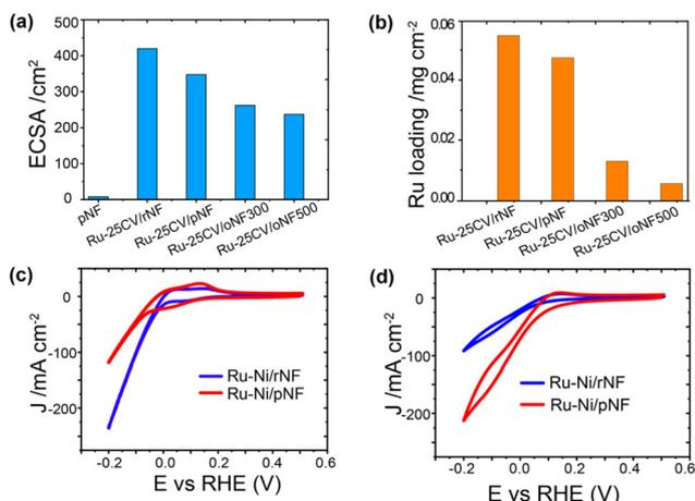
**Fig. 3** (a) The measured ECSA and (b) electrodeposited Ru loading amount on different substrates for 25 CVs deposition. The LSV of Ru-25CV/pNF and Ru-25CV/rNF in Ar saturated (c) 1.0 M KOH and (d) 1.0 M KOH with 0.1 M NaNO<sub>3</sub> at the scan rate of 10 mV s<sup>-1</sup>.
