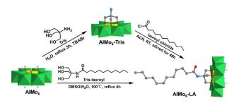
Fig. 8 Synthesis of AlMo<sub>6</sub>-LA by pre- or post-modification methods. Color code: {MoO<sub>6</sub>}, green octahedron; {AlO<sub>6</sub>}, yellow octahedron; C, gray; O, deep red; N, light blue; H, light grey.
