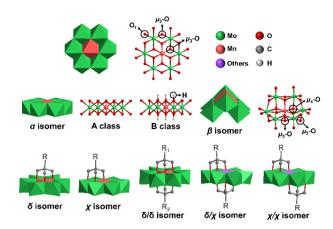
Fig. 1 Structures and isomeric species of Anderson-type POMs, and isomeric species after modification with triol ligands. Color code: {MoO<sub>6</sub>}, green octahedron; {MnO<sub>6</sub>}, red octahedron; {XO<sub>6</sub>}, violet octahedron (X = others). Hydrogen atoms in organic ligands have been omitted for clarity.
