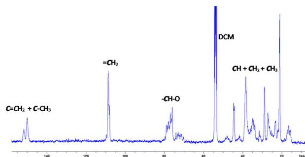
**Fig. 3** <sup>13</sup>C-NMR spectrum of PLO at RT. <sup>13</sup>C-NMR (CD<sub>2</sub>Cl<sub>2</sub>, 400 MHz, RT):  $\delta$  (ppm) = 152.0 (Cq, C–CH–O), 150.0 (Cq, C=CH<sub>2</sub>), 107.4–110.1 (C=CH<sub>2</sub>), 75.0–80.7 (CH–O), 44.5 (CH), 38.4 (CH<sub>2</sub>), 34.4 (CH<sub>2</sub>), 28.9 (CH<sub>2</sub>), 21.2 (CH<sub>3</sub>), and 16.5 (CH<sub>3</sub>).
