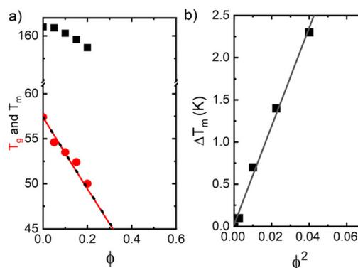
Fig. 5 (a)  $T_g$  (circles) and  $T_{end}$  (squares) compositional dependence in the samples under study. The solid line represents the fit to the Fox equation, and the dashed line the corresponding fit to the Gordon–Taylor approach. (b) Melting temperature depression obtained for the same set of samples. The line represents a linear fit to the Nishi–Wang approach.
