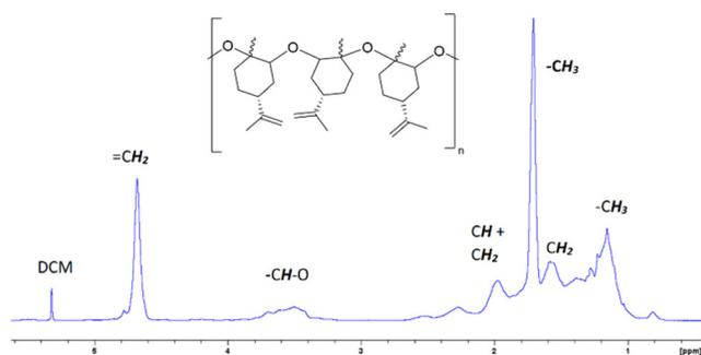
**Fig. 2** <sup>1</sup>H-NMR spectrum of PLO at RT. <sup>1</sup>H-NMR (CD<sub>2</sub>Cl<sub>2</sub>, 400 MHz, RT):  $\delta$  (ppm) = 4.68 (s, 2H, H<sub>2</sub>C=C (LO)), 3.20–3.90 (s, 1H, CH–O (LO)), 2.69 (m, 1H, CH (LO)), 1.96 (m, 1H, CH<sub>2</sub>), 2.17 (m, 1H, CH<sub>2</sub>), 1.97–1.79 (m, 2H, CH<sub>2</sub>), 1.76–1.96 (m, 6H, CH<sub>3</sub>), 1.67 (m, 1H, CH<sub>2</sub>), and 1.55 (m, 1H, CH<sub>2</sub>).
