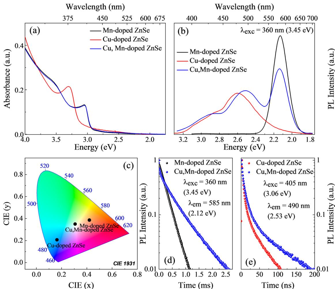
**Fig. 1** Optical characterization of doped ZnSe QDs. (a) UV-visible, and (b) PL spectra of Mn-doped ZnSe (black), Cu-doped ZnSe (red), and Cu, Mn dual-doped ZnSe (blue). (c) Chromaticity diagram showing the CIE coordinates for individually doped as well as dual-doped ZnSe QDs. Comparative decay profile of (d) Mn emission and (e) Cu emission.
