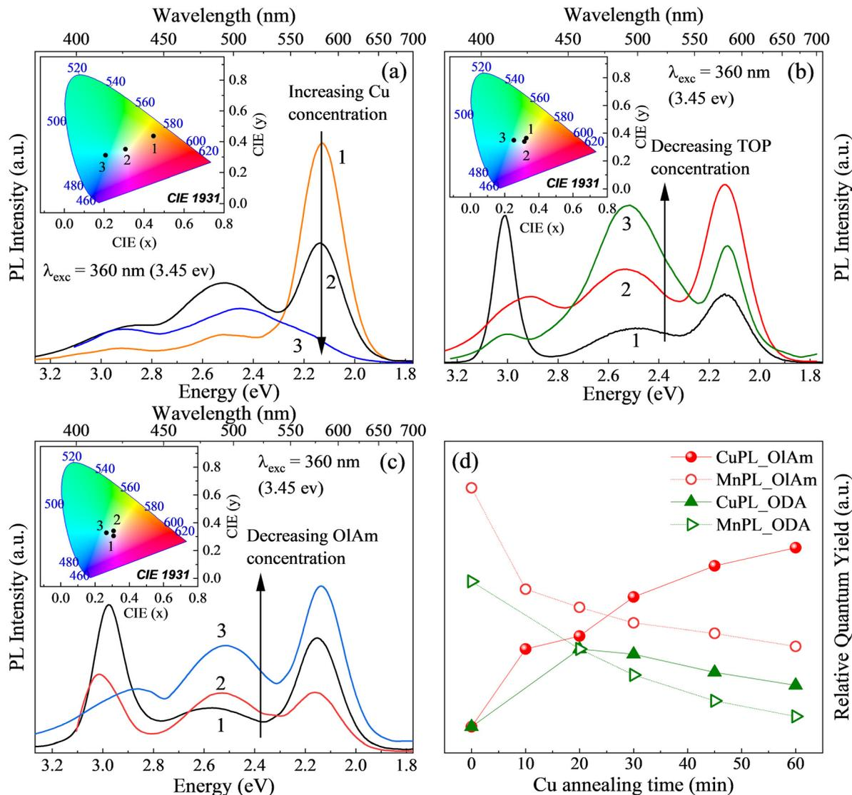
**Fig. 3** PL spectra of Cu, Mn dual-doped ZnSe QDs as a function of (a) Cu concentration (b) TOP concentration, and (c) oleylamine concentration. Corresponding chromaticity diagrams are in the inset to the figures showing the variation in white light emission. (d) Relative quantum yield of Cu (filled shapes) and Mn-related (empty shapes) emission as a function of Cu annealing time when the dual-doped QDs were treated with oleylamine and octadecylamine.
