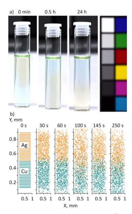
Fig. 10 (a) Photos of the Ag/PEG nanofluid (50  $\mu$ g mL<sup>-1</sup>, 1.5 mL) added on top of the Cu/PEG nanofluid (50 μg mL<sup>-1</sup>, 1.5 mL) without mechanical mixing and left undisturbed for 1 day; experiments are performed 80 days after sample preparation; (b) 2D CFD simulations of collective motion of Ag (orange) and Cu (green) NPs in PEG; Ag/PEG is placed on top of Cu/PEG at time zero.
