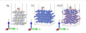
Fig. 11 Relaxed interface geometries of EG onto the Ag(111), Cu(111), and Cu<sub>2</sub>O (111) surfaces.
