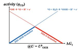
Fig. 1 Generalized volcano plot for the oxygen evolution reaction based on the mononuclear mechanism under equilibrium conditions (U = 1.23 Vvs. RHE). \*OOH and \*O formations are reconciled with the potentialdependent steps (PDS) at the left and right volcano legs, respectively.
