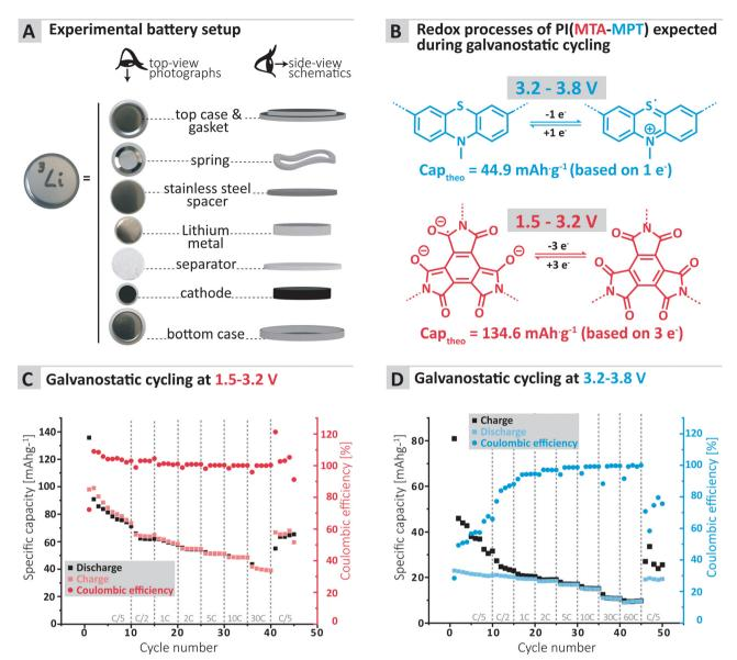
Fig. 3 (A) Experimental setup used to assess the cycling performance of the MTA-MPT porous polyimide as well as (B) the redox mechanism expected to occur for each redox processes during cycling. Galvanostatic cyling of the MTA-MPT porous polyimide in a lithium metal battery at various C-rate with different voltage ranges: (C) 1.5 V-3.2 V (imide process), (D) 3.2-3.8 V (phenothiazine process)
