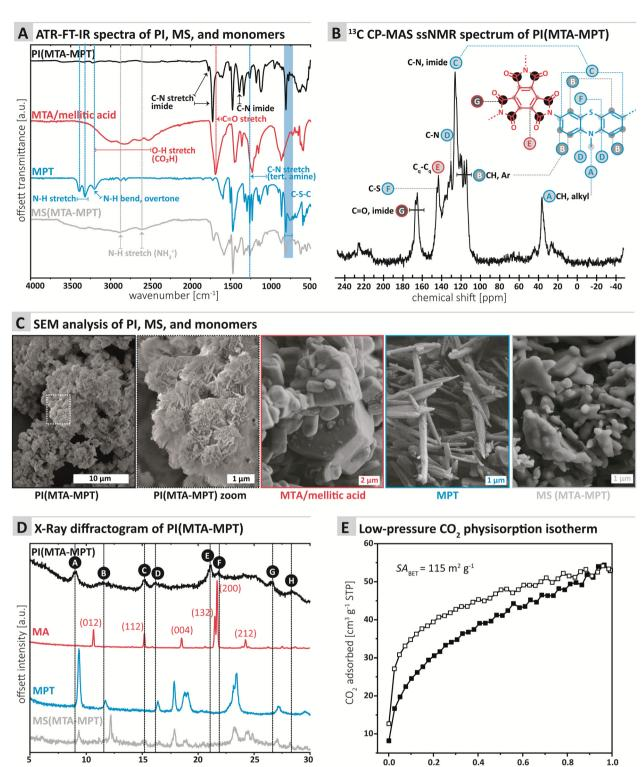
Fig. 1 Characterization of the PI MTA-MTP. (A) ATR-FTIR spectra of PI, monomers, and MS, with mode assignment. (B) 13C CP-MAS solid-state NMR spectrum of PI MTA-MTP with signal assignment. (C) SEM images of PI, monomers, and MS. (D) Powder X-ray diffractogramm of PI, monomers, and MS. (E) Low-pressure CO<sub>2</sub> physisorption isotherm (white squares: adsorption; black squares: desorption).
