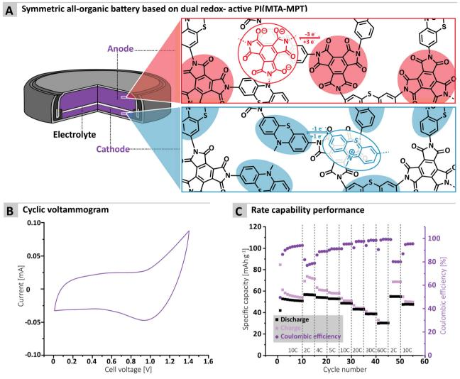
Fig. 5 (A) Scheme illustrating the principle of a symmetric all-organic battery, based on the MTA-MPT porous polymer, (B) cyclic voltammetry of the resulting symmetric all-organic cell as well as (C) its rate capability performance
