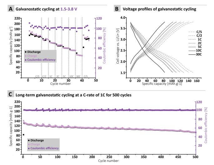
Fig. 4 (A) Galvanostatic cyling of the MTA-MPT porous polyimide in a lithium metal battery at various C-rate with a voltage ranges of 1.5 V-3.8 V (both imide & phenothiazine processes) and (B) its corresponding voltage profile. (C) Long-term cycling at a C-rate of 1C for 500 cycles.
