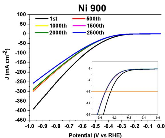
**Fig. 10** HER stability test (2500 cycles) on the Ni 900 electrocatalyst.
