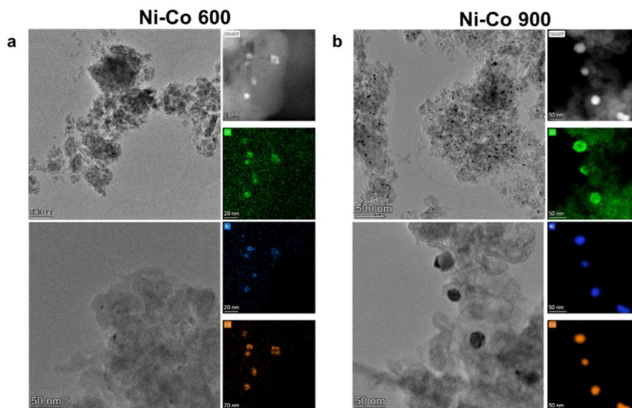
**Fig. 2** (a) TEM characterization of the Ni-Co 600 °C and Ni-Co 900 °C samples. For each sample, leftmost top image and bottom image report HRTEM characterization, while the rightmost column reports the STEM EDX mapping. (a) The Ni-Co sample functionalized at 600 °C (Ni-Co 600), and (b) the sample functionalized at 900 °C (Ni-Co 900).
