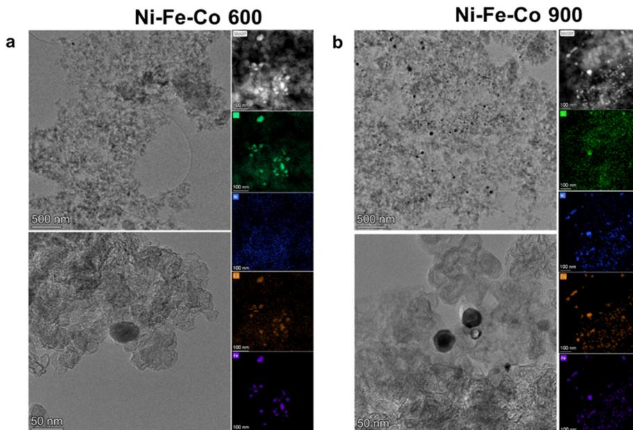
**Fig. 3** (a) TEM characterization of the Ni-Fe-Co 600 °C and Ni-Fe-Co 900 °C samples. For each sample, leftmost top image and bottom image report HRTEM characterization, while the rightmost column reports the STEM EDX mapping. (a) The Ni-Fe-Co sample functionalized at 600 °C (Ni-Fe-Co 600), and (b) the sample functionalized at 900 °C (Ni-Fe-Co 900).
