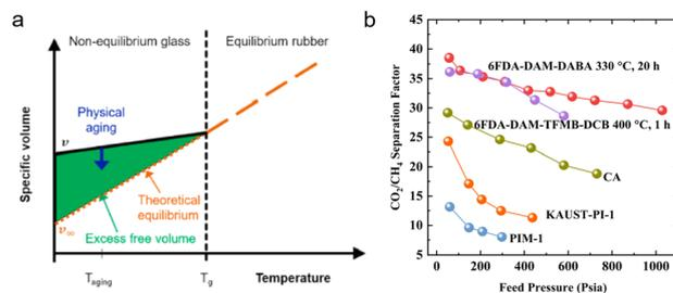
Fig. 5 (a) Physical aging of amorphous polymers (reprinted with permission from ref. 66, Copyright (2020) Elsevier) and (b) plasticization of typical crosslinked polyimide and PIM membranes (reprinted with permission from ref. 67, Copyright (2023) American Chemical Society).
