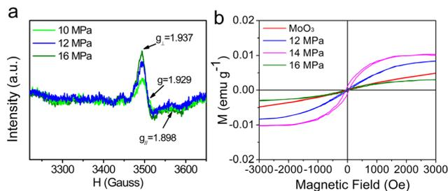
Fig. 6 (a) EPR spectra comparison of  $\text{MoO}_{3-x}$  obtained at different pressures; (b) magnetization hysteresis loop comparison of the  $\text{MoO}_{3-x}$  sample obtained at 12 MPa, 14 MPa, 16 MPa and crystalline  $\text{MoO}_3$  at 300 K.
