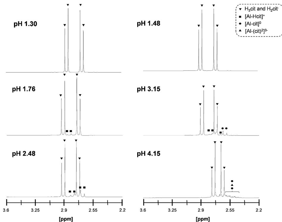
Fig. 4  $^1\text{H}$ -NMR spectra of mixtures containing 0.1 M of citric acid and 0.25 eq.  $\text{Al}_2(\text{SO}_4)_3$  at different pH levels: pH 1.30 (0.5 eq.  $\text{H}_2\text{SO}_4$ ), pH 1.48 (1 eq.  $\text{H}_2\text{SO}_4$ ), pH 1.76 (no additive), pH 2.48 (0.5 eq.  $\text{NaOH}$ ), pH 3.15 (1 eq.  $\text{NaOH}$ ) and pH 4.15 (2 eq.  $\text{NaOH}$ ).<sup>50,51,56</sup>
