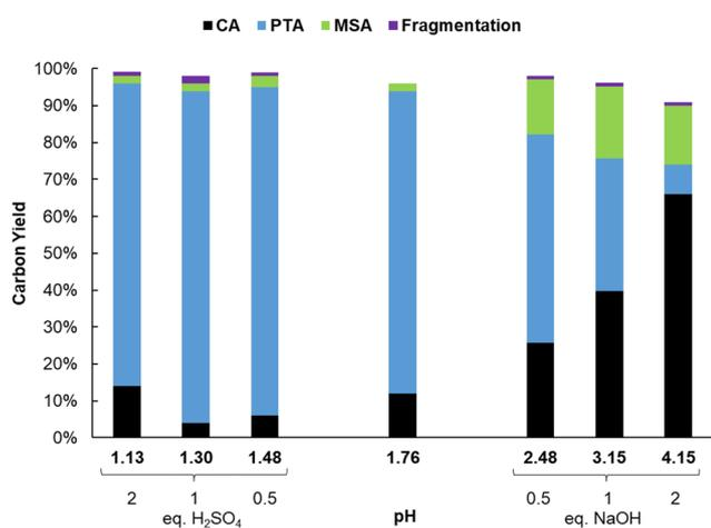
Fig. 1 Dehydration-hydrogenation of citric acid. Reaction in water (2 mL) with citric acid (0.2 mmol), Al<sub>2</sub>(SO<sub>4</sub>)<sub>3</sub> (0.05 mmol), Pd<sup>0</sup>/C (0.5 mol% Pd<sup>0</sup>), 20 h with 10 bar H<sub>2</sub> at 150 °C. Different amounts (0.5; 1 and 2 equivalents) of H<sub>2</sub>SO<sub>4</sub> and NaOH.
