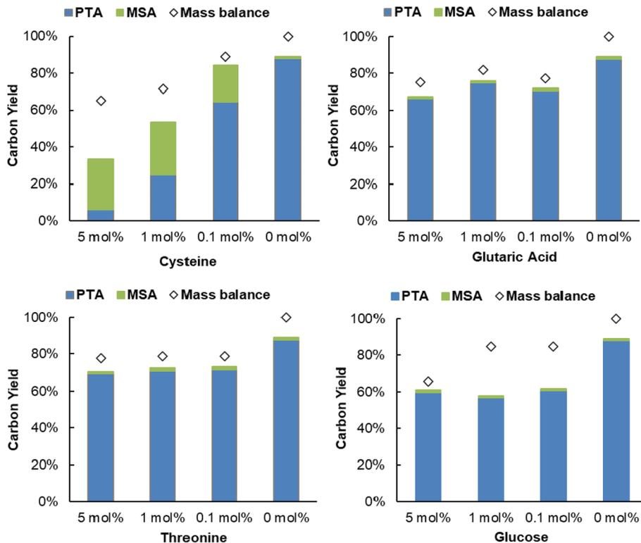
Fig. 7 Influence of amino acids with different functional groups ( $-\text{SH}$ ,  $-\text{OH}$ ,  $-\text{COOH}$ ) and glucose on dehydration-hydrogenation of citric acid. Reaction in water (2 mL) with citric acid (2 mmol),  $\text{Al}_2(\text{SO}_4)_3$  (0.25 mmol),  $\text{Pd}^0/\text{C}$  (0.5 mol%  $\text{Pd}^0$ ), 20 h with 20 bar  $\text{H}_2$  at 150 °C.
