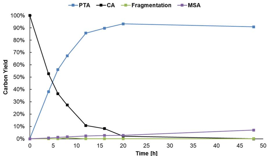
**Fig. 6** Time profile of the dehydration-hydrogenation of citric acid. Reaction in water (20 mL) with citric acid (20 mmol),  $\text{Al}_2(\text{SO}_4)_3$  (1.25 mmol),  $\text{Pd}^0/\text{C}$  (0.5 mol%  $\text{Pd}^0$ ) with 20 bar  $\text{H}_2$  at 150 °C.
