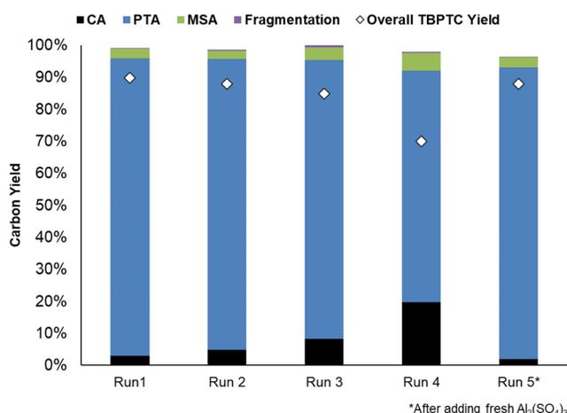
**Fig. 9** Recycling of the catalytic system (*i.e.*  $\text{Pd}^0/\text{C}$  and  $\text{Al}_2(\text{SO}_4)_3$ ) for the two-step process. Reaction in water (20 mL) with citric acid (20 mmol),  $\text{Al}_2(\text{SO}_4)_3$  (1.25 mmol),  $\text{Pd}^0/\text{C}$  (0.5 mol%  $\text{Pd}^0$ ), 20 h with 20 bar  $\text{H}_2$  at 150 °C.
