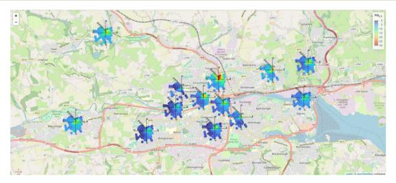
Fig. 10 Polar plots showing associations between wind speed and direction, and local PM<sub>2.5</sub> levels at the locations monitored in the sensor network.
